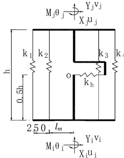
Fig.2 Macro-model of GFRP with fully filled with reinforced concrete
