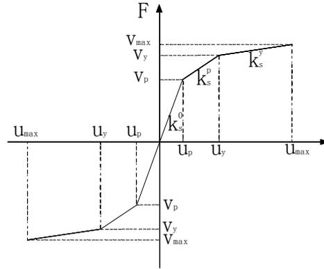
Fig.5 Skeleton curve of horizontal spring
