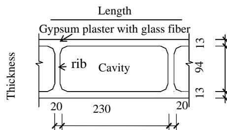
Fig.1. Cross section of a GFRGP
