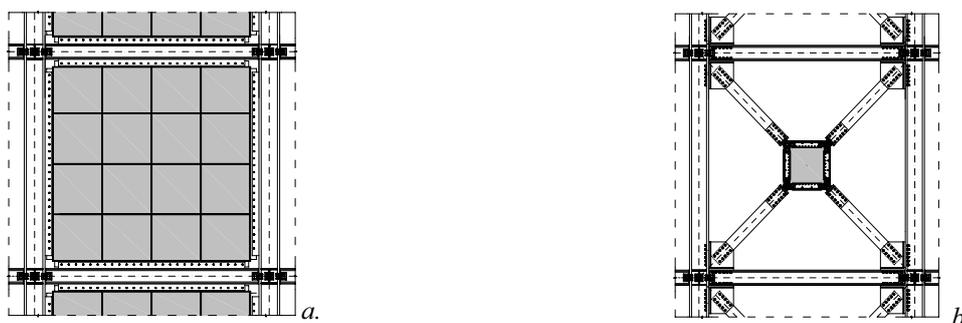
Figure 1: Shear panel typologies installed into a framed steel structure: (a) full bay type and (b) bracing type.
