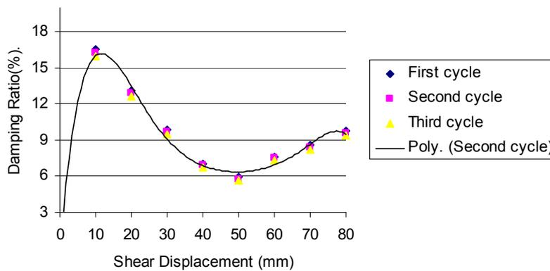
Figure 10 Shear effective damping ratio-displacement relation
