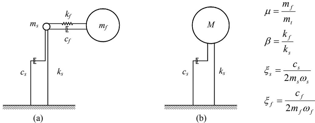
Figure 2 Analytical models of one-story shear building (a) with FIS (b) without FIS
