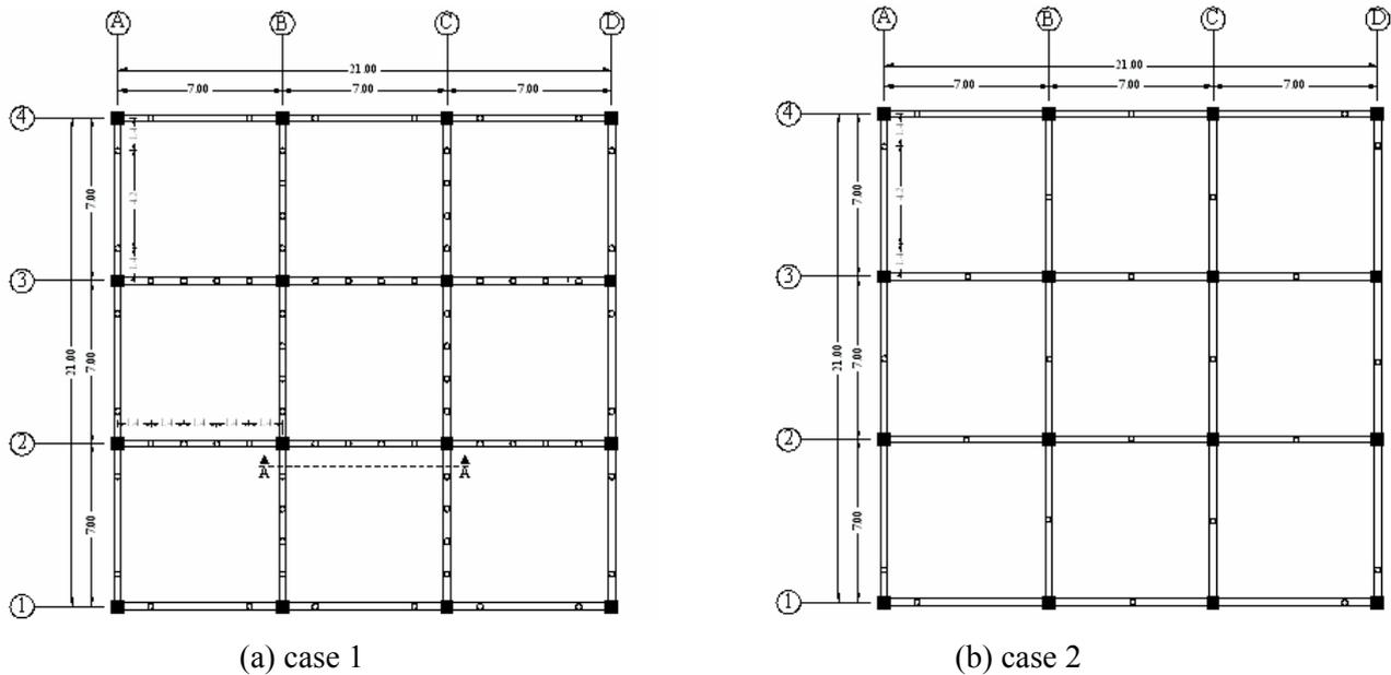
Figure 4. Isolators locations on beams for each story
