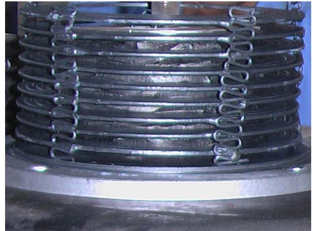
a) Inner steel rings with assembling plain bars
