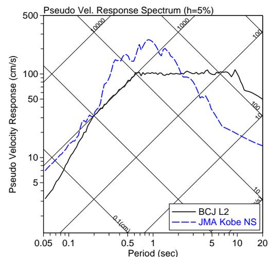
Fig.10 Tripartite response spectra of input ground motions
