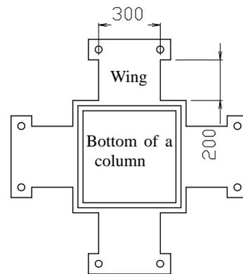
Fig.4 Plan of yielding base plate
