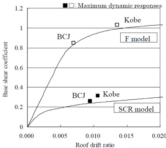
Fig.11 Relationship between roof displacement and base shear obtained by static pushover analysis and corresponding maximum dynamic responses.
