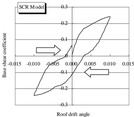
Fig.18 Relationship between roof displacement and base shear for static cyclic load of SCR model
