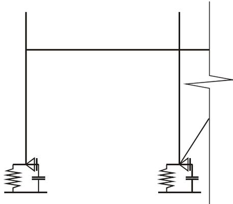
Fig.6 Column bases with two types of springs
