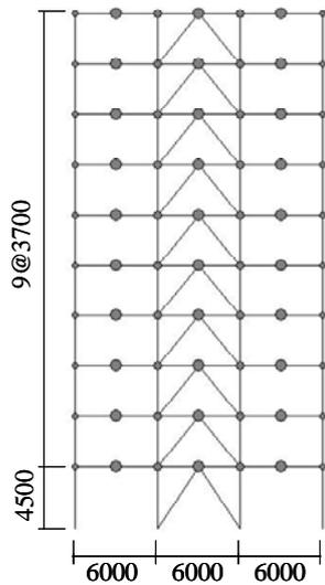
Fig.2 Braced frame model with fixed bases
