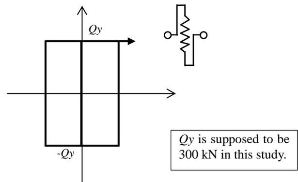
Fig.9 Force-deformation relation of vertical dampers used in coupled brace unit
