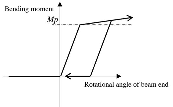
Fig.8 Force-deformation relation of one-side rocking beam
