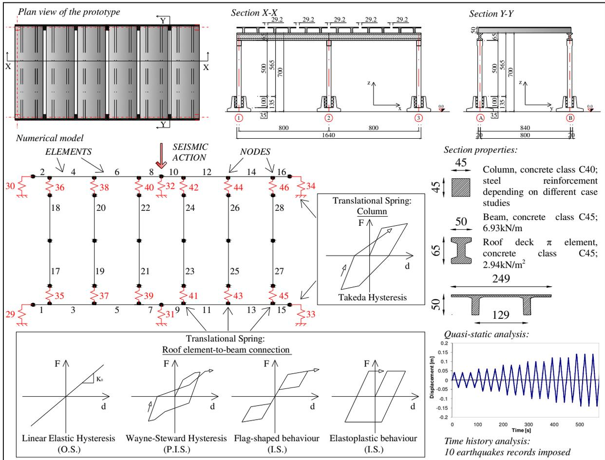
Figure 6 – Experimental prototype and numerical model
