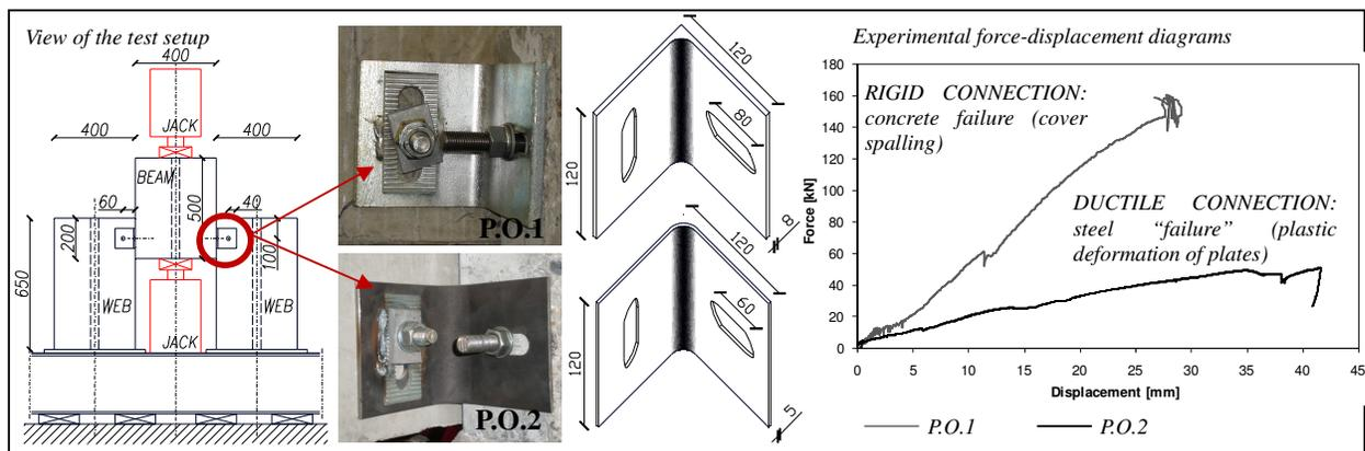
Figure 4 – Push-over test: comparison of two different connections’ behaviour
