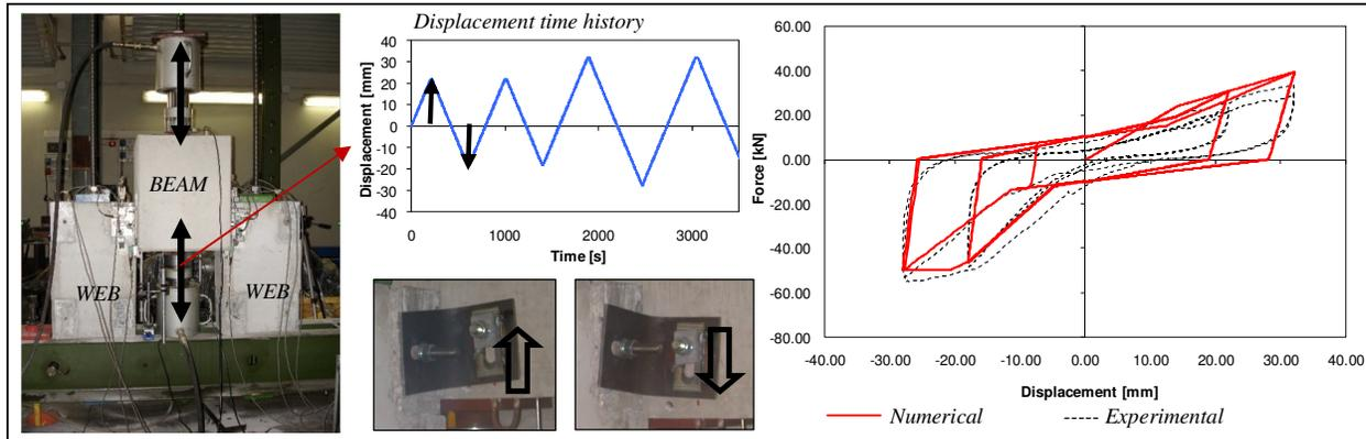
Figure 5 – Cyclic test: experimental-numerical comparison of force-displacement diagrams
