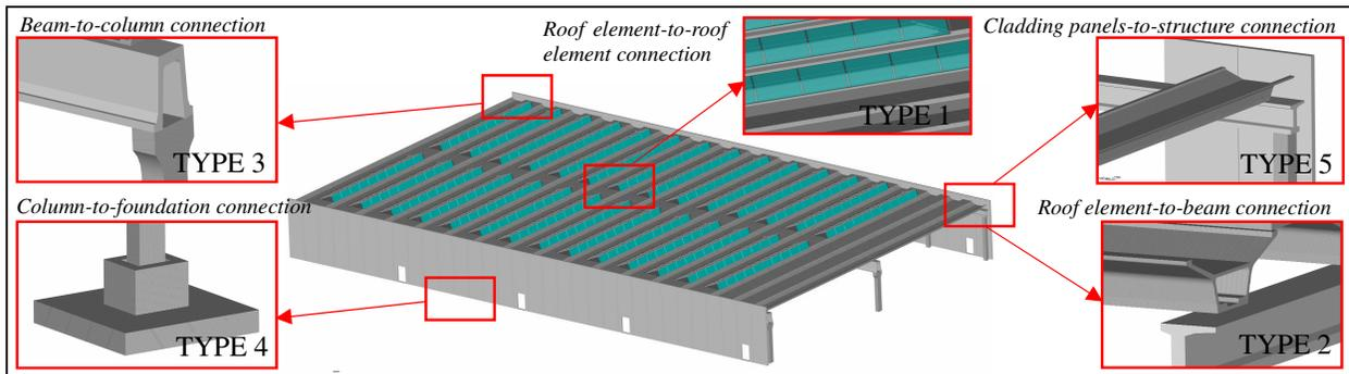
Figure 1 – Different typologies of connections between structural members
