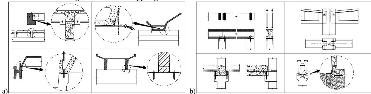
Figure 2 – a) Roof element-to-beam connections; b) Beam-to-column connections
