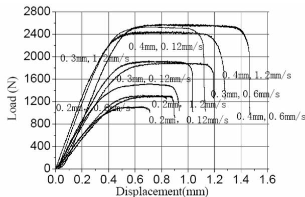
Figure 1: Relationship between displacement and loading of copperplate
