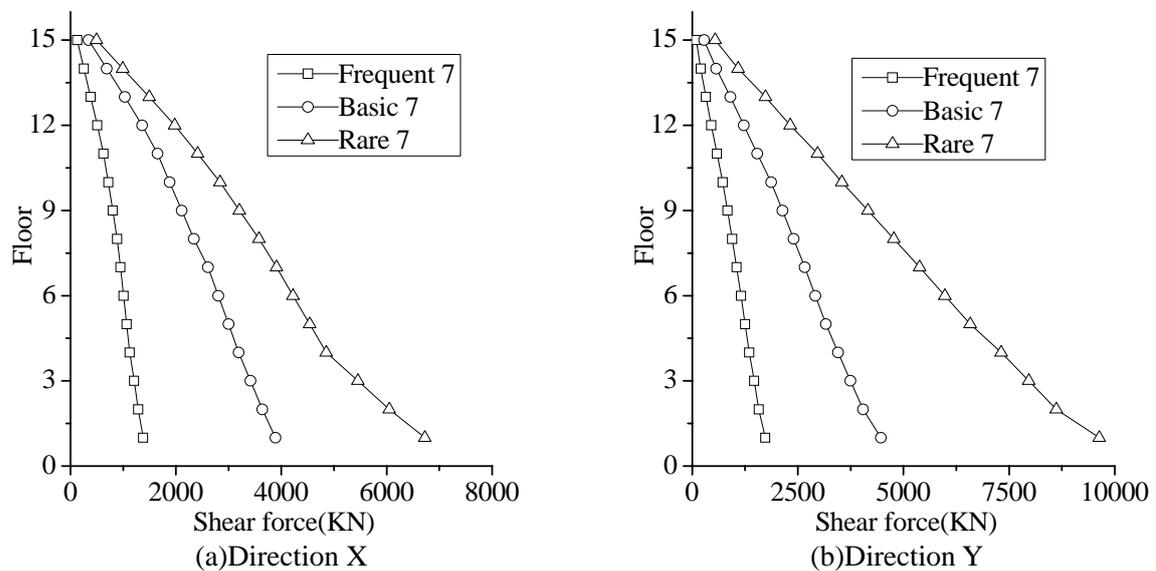
Figure 6: Shear force distribution of the prototype
