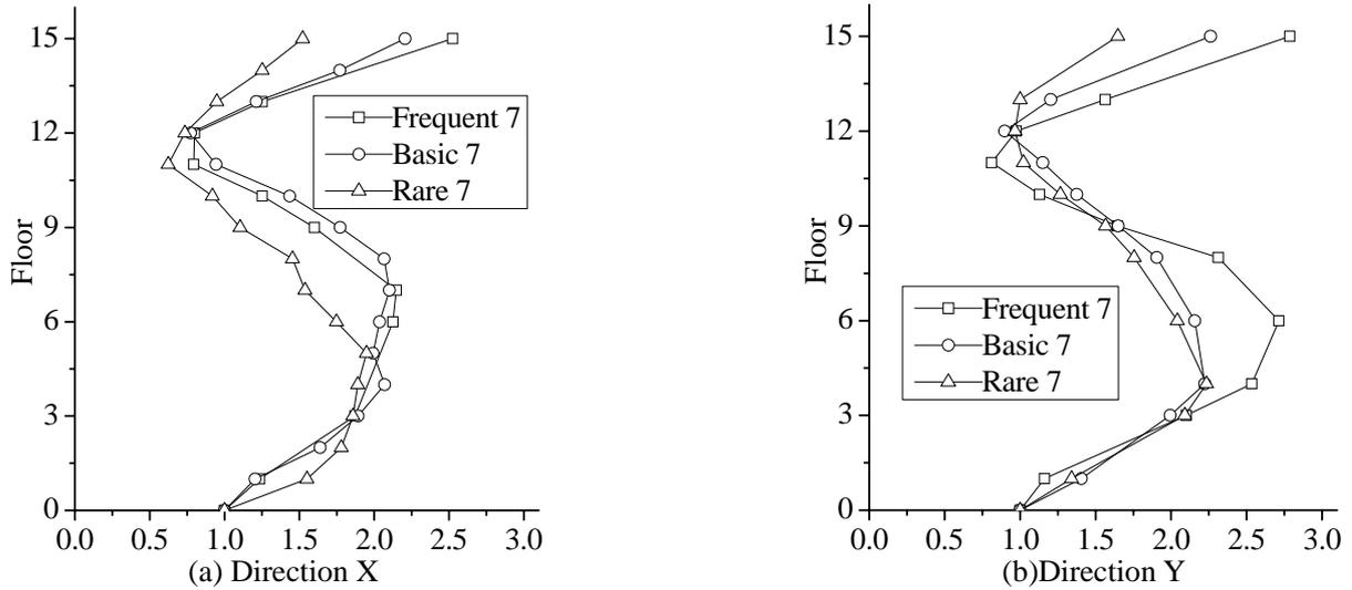
Figure 4: Displacement of the prototype
