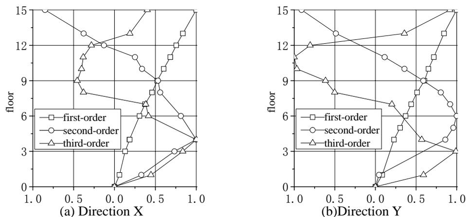
Figure 3: Vibration mode of the prototype
