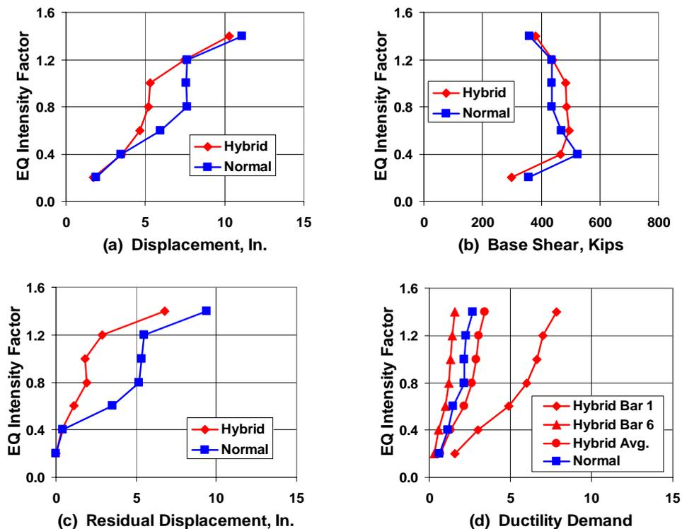
Figure 4 - Results of Frame Analysis With P-Delta Analysis
