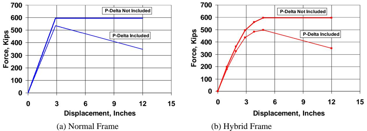
**Figure 2 - Nonlinear Static Pushover Curves for Braced Frame Structure**
