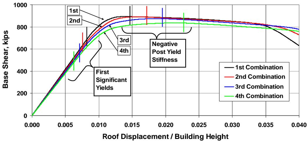
Figure 6 - Static Pushover Curves for Hybrid Frames
