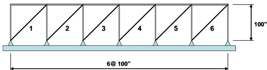
Figure 1 - A Simple Braced Frame
