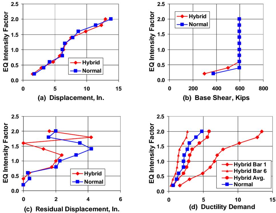
Figure 3 - Results of Frame Analysis Without P-Delta Analysis
