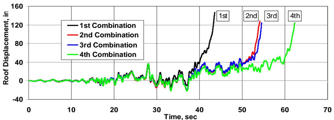
Figure 8 - Roof Displacement Response History of Hybrid Frames subject to Valpariso Earthquake with scale of 1.8 times the anchored design spectrum scale.
