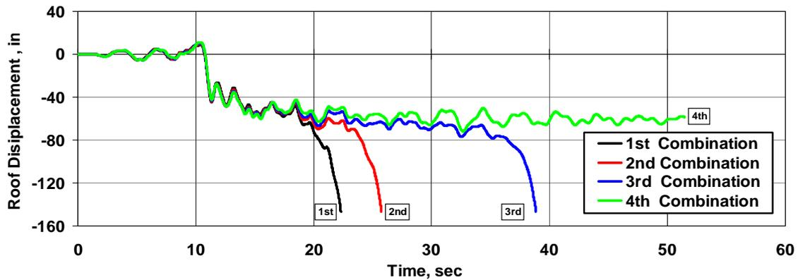
Figure 7 - Roof Displacement Response History of Hybrid Frames subject to Miyagi Oki Earthquake with scale of 2.0 times the anchored design spectrum scale.
