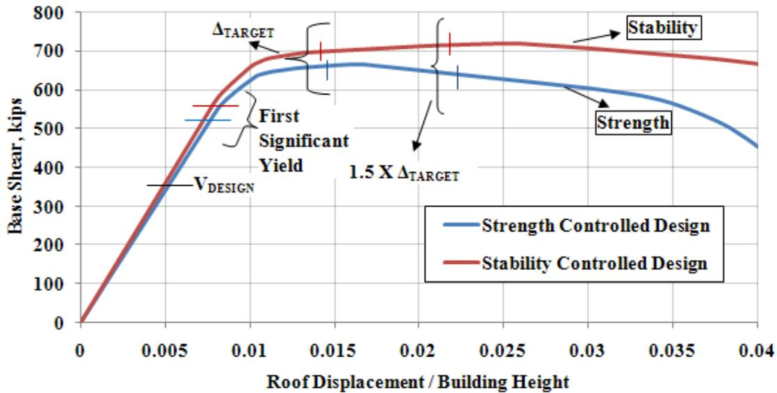
Figure 2. Nonlinear static pushover curves for strength and stability controlled designs
