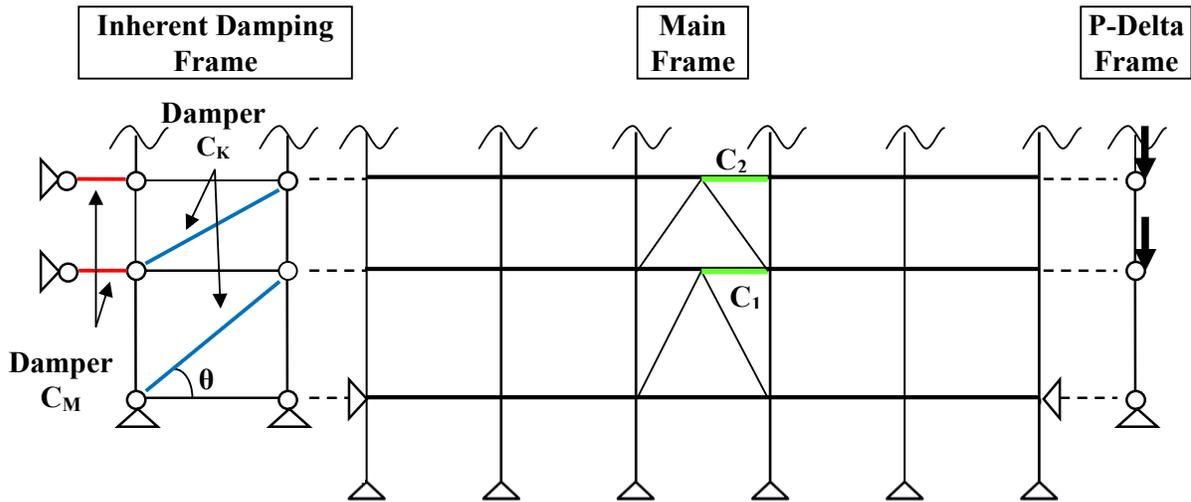
Figure 1. Inherent Damping and P-Delta Frames Constrained to Main Frame
