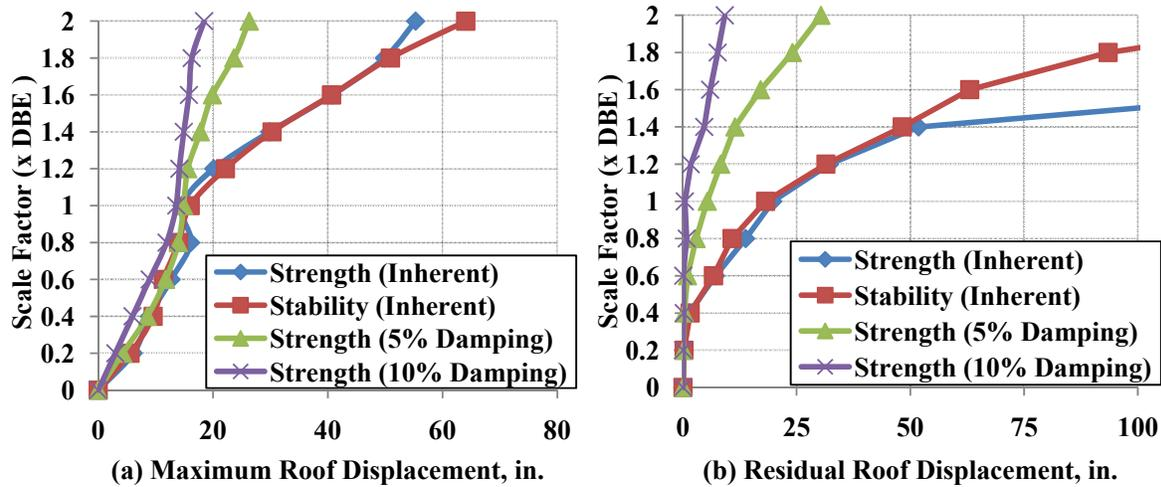
Figure 3. IDA plots for Maximum and Residual Roof Displacements using Valpariso-1 and Seattle Eq.
