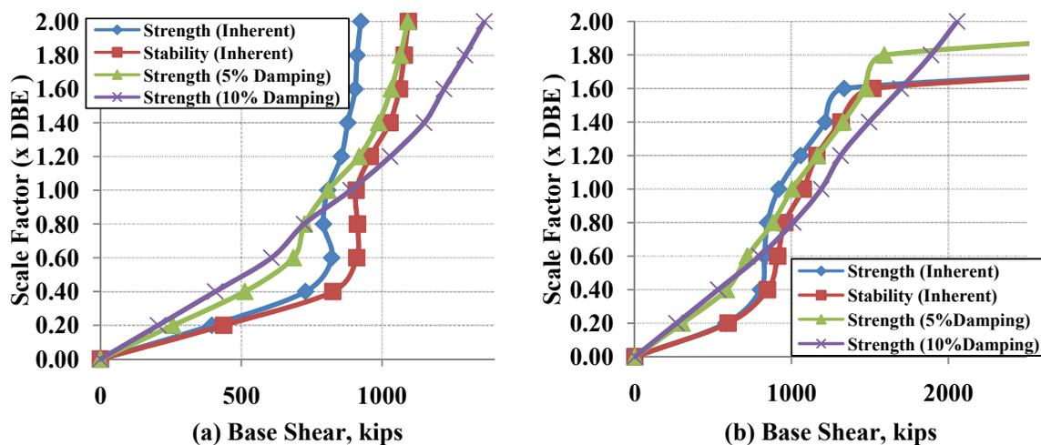
Figure 4 Base Shear IDA Plots for Erzincan (a) and Miyagi Oki (b) Earthquakes
