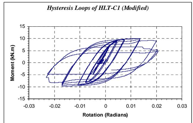
Figure 18- The 'modified' hysteresis loops of an 'average' connection of the first test assembly, HLT-C1.
