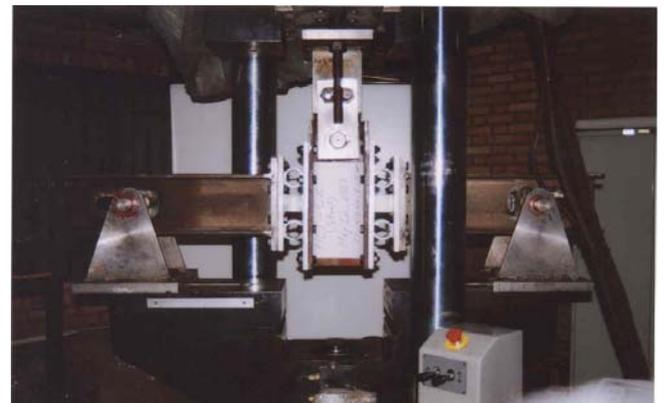
Figure 11- Second test assembly, with HLT-C2 specimens, before the test.
