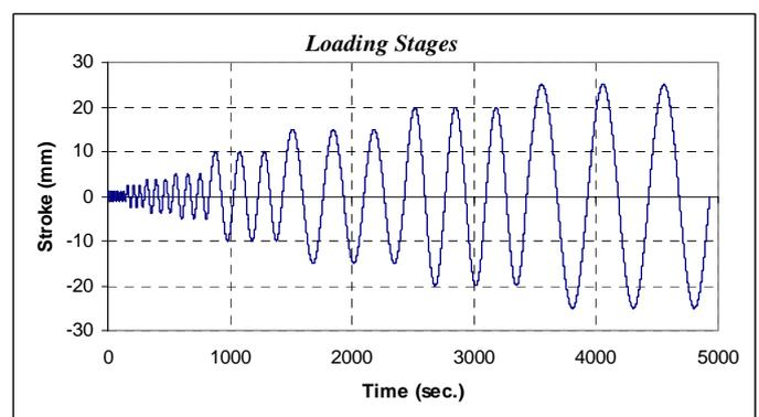
Figure 7- The variation of amplitude of the stroke, given to the Universal Testing Machine for test assemblies with HLT-C2 and HLT-C3 specimens.
