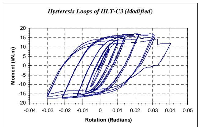
Figure 22- The 'modified' hysteresis loops of an 'average' connection of the third test assembly, HLT-C3.
