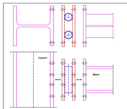
Figure 2- The Vertically-Laid-Tubes (VLT) version of KHONSAR™ with just high ‘rotational’ deformation capacity.
