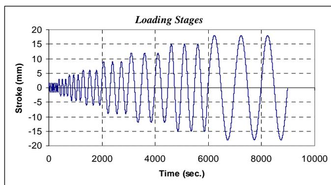
Figure 6- The variation of amplitude of the stroke, given to the Universal Testing Machine for test assembly with HLTC1 specimens.
