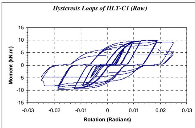
Figure 17- The 'raw' hysteresis loops of an 'average' connection of the first test assembly, HLT-C1.
