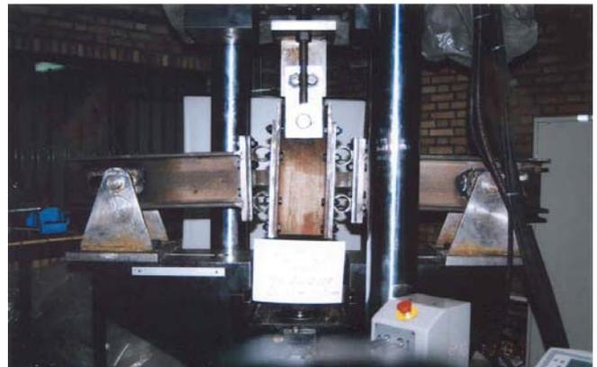
Figure 15- Third test assembly, with HLT-C3 specimens, at its utmost upper position, before failure.
