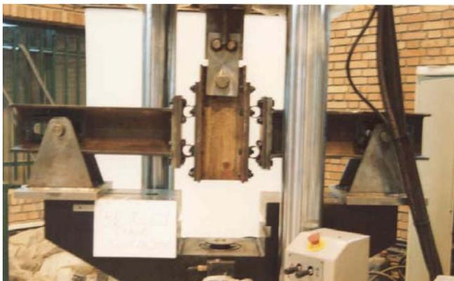
Figure 8- First test assembly, with HLT-C1 specimens, before the test.
