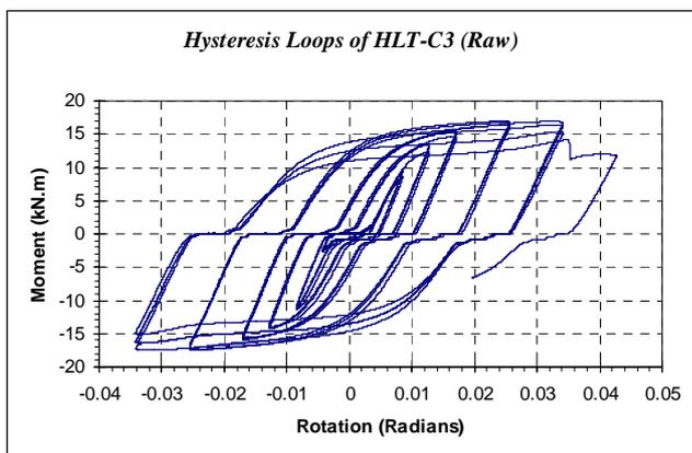
Figure 21- The 'raw' hysteresis loops of an 'average' connection of the third test assembly, HLT-C3.
