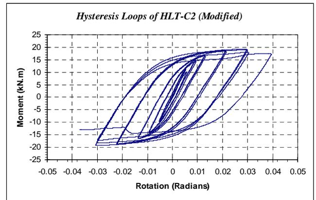
Figure 20- The 'modified' hysteresis loops of an 'average' connection of the second test assembly, HLT-C2.
