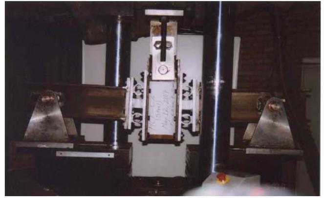
Figure 13- Second test assembly, with HLT-C2 specimens, at its utmost lower position, before failure.
