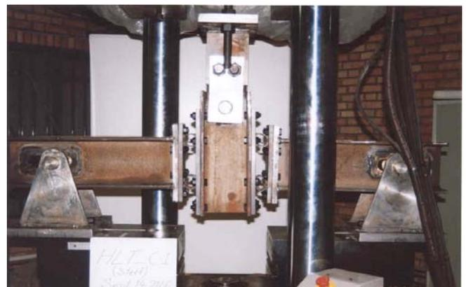
Figure 9- First test assembly, with HLT-C1 specimens, at its utmost upper position, before failure.
