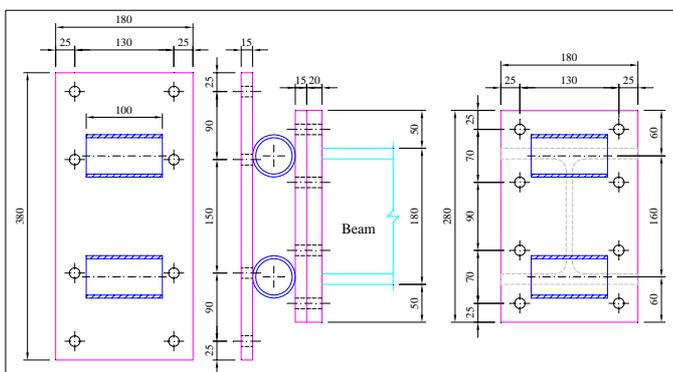
Figure 4- Details of the specimens HLT-C1 of KHONSAR™ connection.
