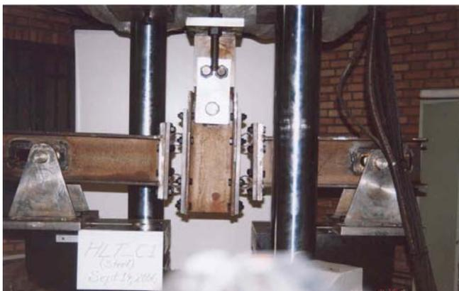
Figure 10- First test assembly, with HLT-C1 specimens, at its utmost lower position, before failure.
