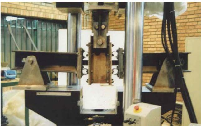
Figure 16- Third test assembly, with HLT-C3 specimens, at its utmost lower position, before failure.
