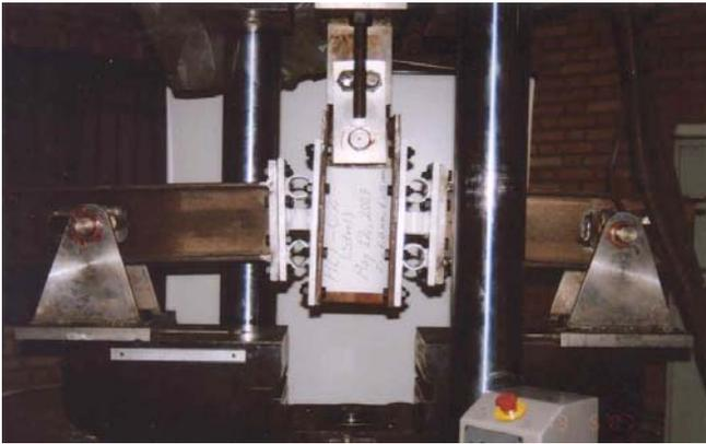
Figure 12- Second test assembly, with HLT-C2 specimens, at its utmost upper position, before failure.
