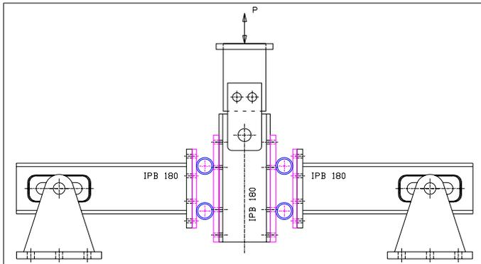
Figure 3- The test assembly designed and fabricated to enable the authors to apply cyclic loading to the specimens of the connection through UTM. IPB180 is a mid-weight wide flange section with 180 mm height and 180 mm width, based on DIN standard.
