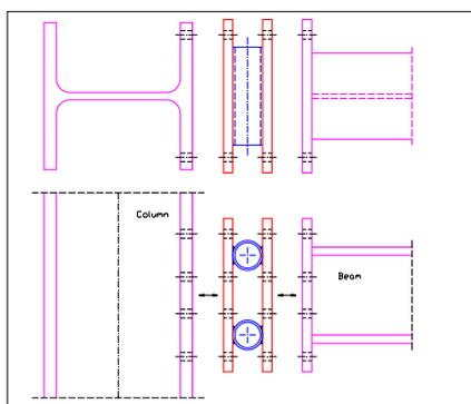
Figure 1- The Horizontally-Laid-Tubes (HLT) version of KHONSAR™, with high ‘rotational’ as well as ‘shear’ deformation capacity.
