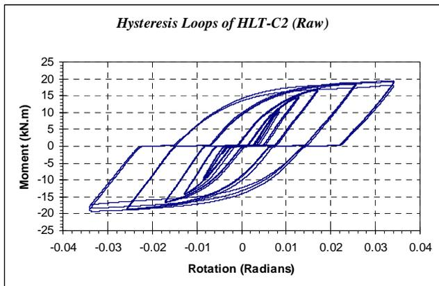
Figure 19- The 'raw' hysteresis loops of an 'average' connection of the second test assembly, HLT-C2.
