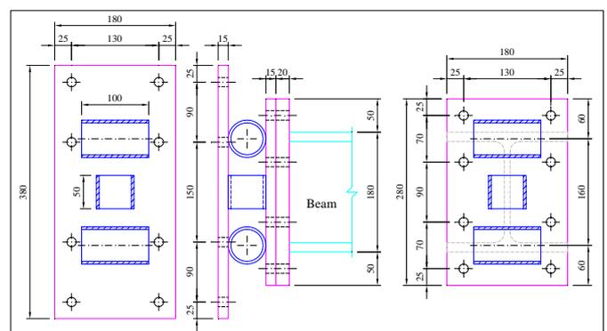
Figure 5- Details of the specimens HLT-C2 & HLT-C3 of KHONSAR™ connection.
