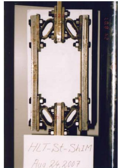
Figure 6- First series of monotonically tested specimens, HLT-St-Sh-1-M, after the test.
