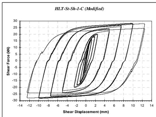
Figure 21- Hysteresis loops of an 'average' tube of the 1st cyclically loaded test assembly, HLT-St-Sh-1-C, before serious strength degradation starts.
