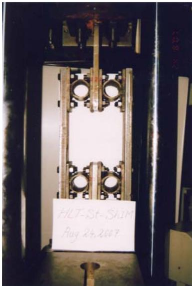
Figure 4- First series of monotonically tested specimens, HLT-St-Sh-1-M, before the test.
