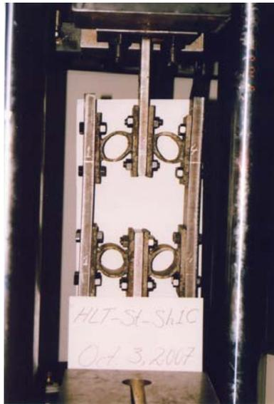
Figure 14- First series of specimens tested under cyclic loading, HLT-St-Sh-1-C, at the most overall tensile state.
