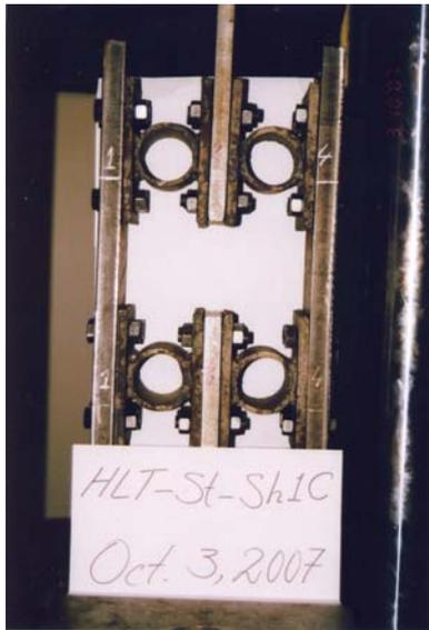
Figure 13- First series of specimens tested under cyclic loading, HLT-St-Sh-1-C, before loading.
