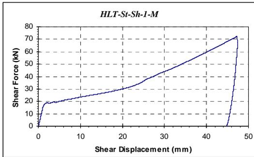
Fig. 10- 'Average' Shear Force-Shear Displacement curve of one of the tubes of the 1st test assembly, HLT-St-Sh-1-M, tested under monotonic loading.
