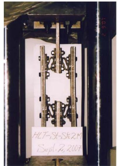
Figure 9- Second series of monotonically tested specimens, HLT-St-Sh-2-M, after the test.
