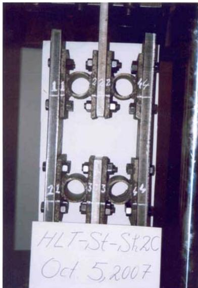
Figure 16- Second series of specimens tested under cyclic loading, HLT-St-Sh-2-C, before loading.
