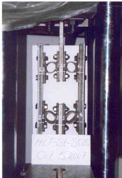
Figure 17- Second series of specimens tested under cyclic loading, HLT-St-Sh-2-C, at the most overall tensile state.
