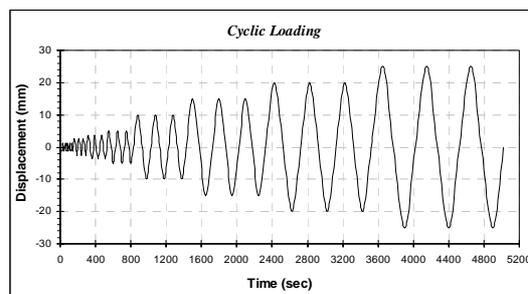
Figure 12- The variation of amplitude of shear deformation of each tube with time, given to the Universal Testing Machine (the amplitude of the crosshead was double this amount).
