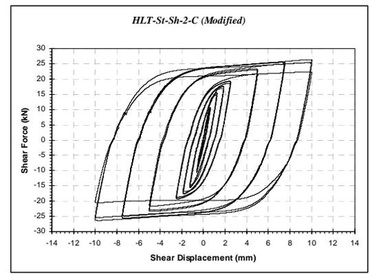
Figure 22- Hysteresis loops of an 'average' tube of the 2nd cyclically loaded test assembly, HLT-St-Sh-2-C, before serious strength degradation starts.
