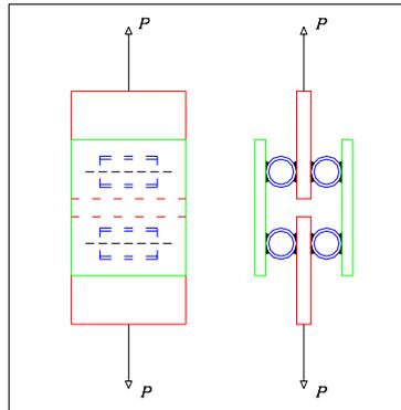
Figure 3- The modified test assembly, applicable to both ‘monotonic’ and ‘cyclic’ tests.
