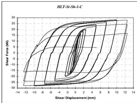
Figure 19- Hysteresis loops of an 'average' tube of the 1st cyclically loaded test assembly, HLT-St-Sh-1-C.
