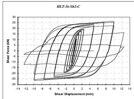
Figure 20- Hysteresis loops of an 'average' tube of the 2nd cyclically loaded test assembly, HLT-St-Sh-2-C.
