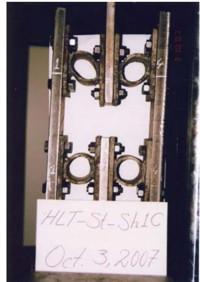
Figure 15- First series of specimens tested under cyclic loading, HLT-St-Sh-1-C, at the most overall compressive state.
