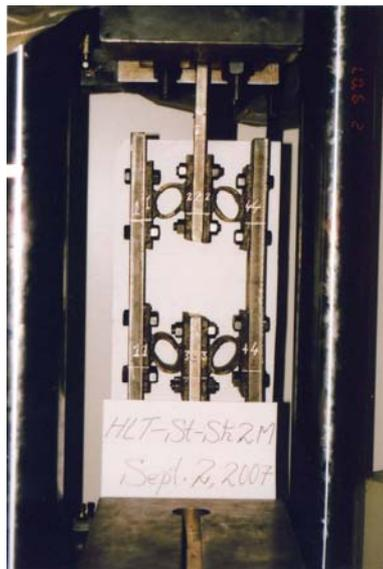
Figure 8- Second series of monotonically tested specimens, HLT-St-Sh-2-M, at the middle of the test.
