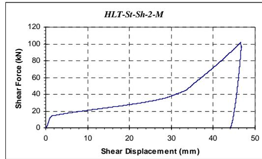
Fig. 11- 'Average' Shear Force-Shear Displacement curve of one of the tubes of the 2nd test assembly, HLT-St-Sh-2-M, tested under monotonic loading.
