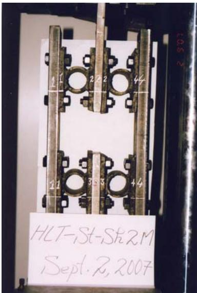
Figure 7- Second series of monotonically tested specimens, HLT-St-Sh-2-M, before the test.
