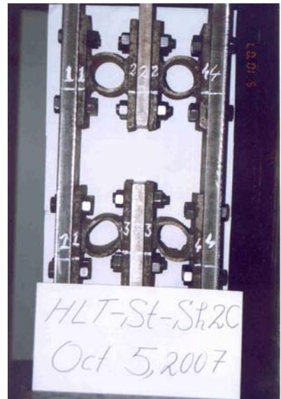
Figure 18- Second series of specimens tested under cyclic loading, HLT-St-Sh-2-C, at the most overall compressive state.
