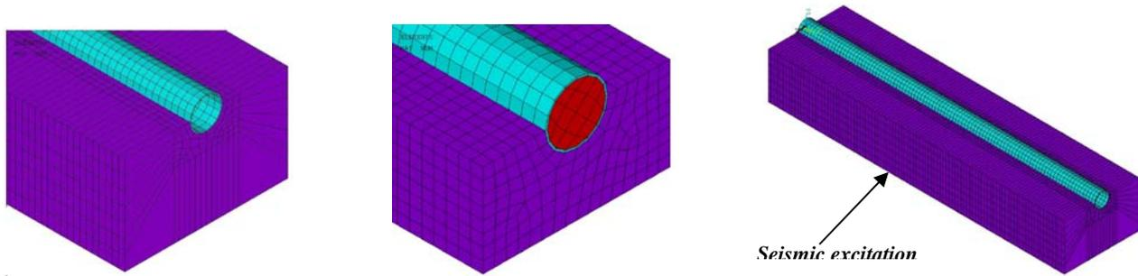
Numerical model of soil-pipeline interaction (*semi-buried pipe*)
