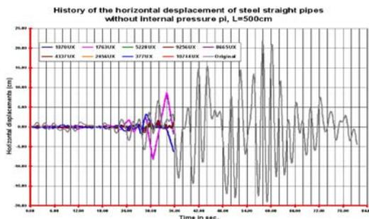
Figure 13.c. - History of the horizontal displacements of the steel pipes segment to  $L_2=500\text{cm}$
