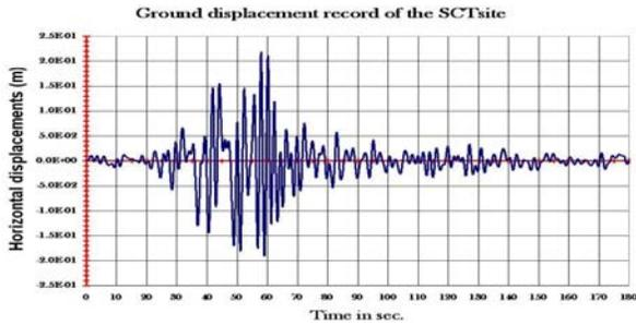
Figure 9 Input seismic displacement record
