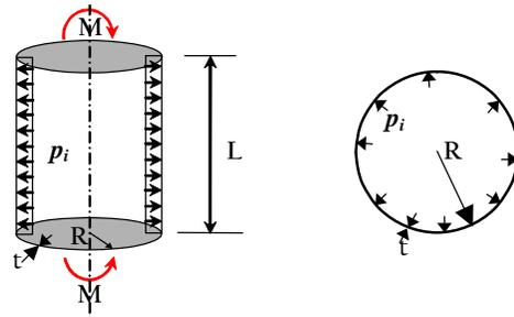
Figure 2 Segment buried steel pipe studied, using a typical steel pipe with 20" external diameter, API 5L X52 (L=10m), submitted to combined mechanical actions
