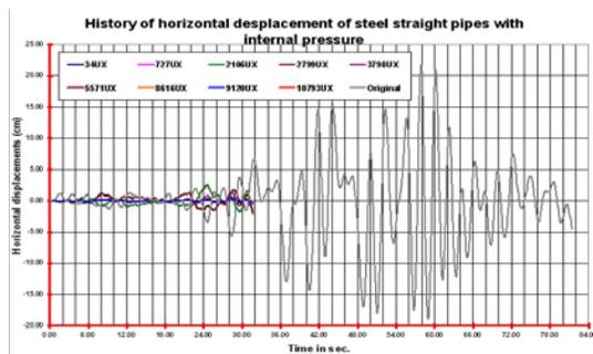
Figure 12.a. – History of the horizontal displacement of the steel pipes segment to  $L_1=10$ cm
