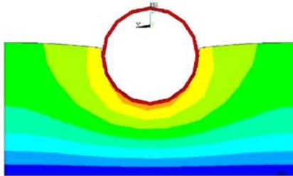
Figure 6.a Numerical model 1 of soil-pipeline interaction of the semi-buried pipe
