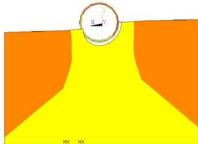
Case a, seismic response of the horizontal displacement
