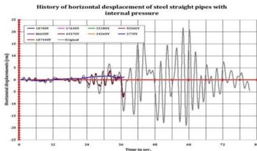
Figure 14.c. History of the horizontal displacements of the steel pipes segment to  $L_2=500\text{cm}$
