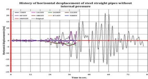
Figure 14.c. History of the horizontal displacements of the steel pipes segment to  $L_3=990cm$
