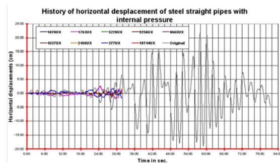
Figure 12.b. – History of the horizontal displacement of the steel pipes segment to  $L_2=500$ cm
