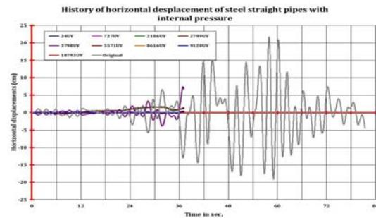
Figure 14.b. History of the horizontal displacements of the steel pipes segment to  $L_1=10\text{cm}$
