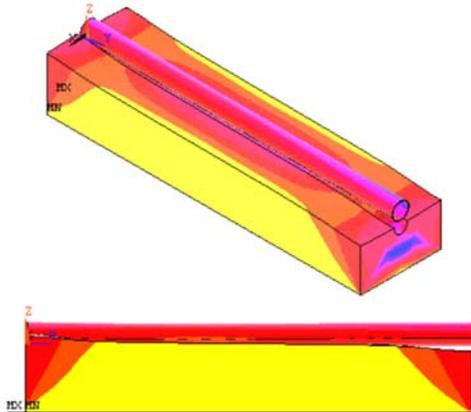
Figure 14.a Case d, 3D and elevation views of the seismic response of the longitudinal displacement
