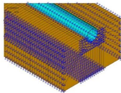
Figure 3.b Boundary conditions of the numerical model of soil-pipeline interaction considering the semi-buried pipe
