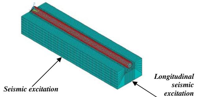
Figure 10 Soil-pipeline interaction numerical model, L=10m
