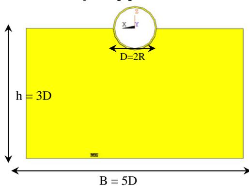
Figure 3.a Geometrical characteristics of the numerical models of soil-pipeline interaction:  $b=5D$ ,  $h=3D$ ,  $L=10m$
