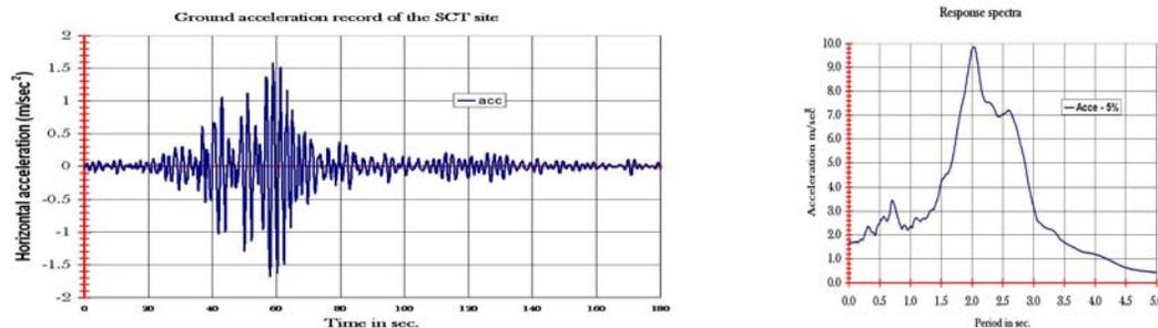
Figure 8 Horizontal ground acceleration record and response spectra, Mexico City
