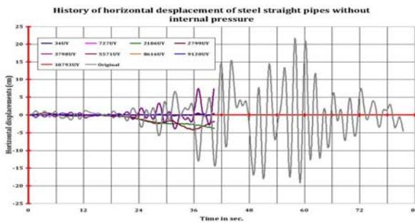
Figure 14.a History of the horizontal displacements of the steel pipes segment to  $L_1=10cm$
