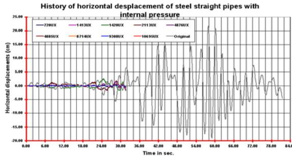
Figure 12.c. – History of the horizontal displacement of the steel pipes segment to  $L_3=990\text{cm}$
