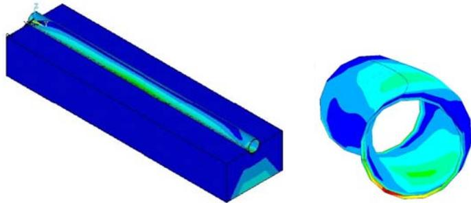
Figure 13.f. - View 3D of the seismic response of the Von Mises stresses of the soil-pipeline interaction model, without  $p_i$
