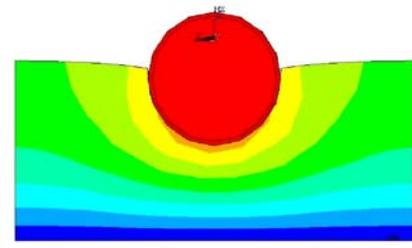
Figure 6.c Numerical model 3 of soil-pipeline-fluid interaction of the semi-buried pipe
