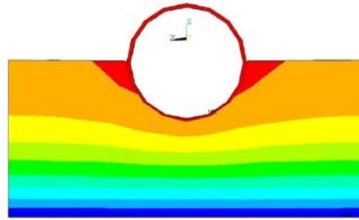
Figure 6.b Numerical model 2 of soil-pipeline interaction of the semi-buried pipe, without fluid
