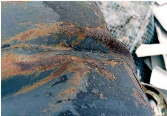
Figure 1 Buried pipe damage by ground shaking effects
