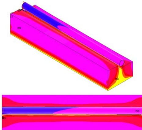
Figure 13.a - 3D and plane view of the seismic response of the transversal displacement
