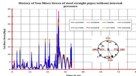
Figure 14.d. History of the Von Mises stresses of the steel pipes without pressure
