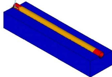
Figure 12.d. View 3D of the seismic response of the Von Mises stresses of the soil-pipeline interaction model, pressure  $p_i = 5.89\text{Mpa}$
