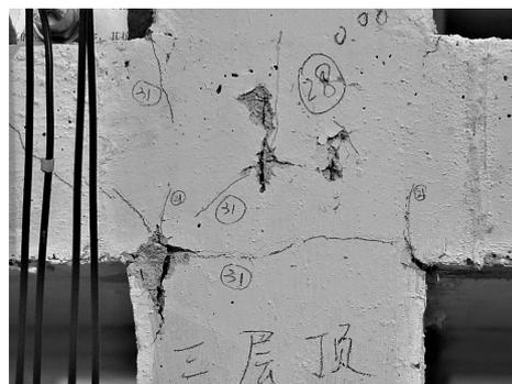
Figure 6 Cracks cross the core of joints in floor 3
