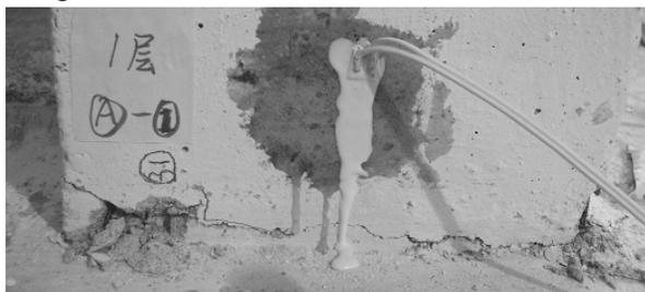
Figure 9 Crack after the input of two bi-direction Taft records of rare intensity
