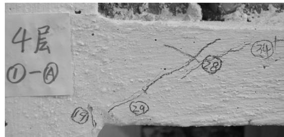
Figure 8 Crack after input of two bi-direction El Centro records of rare intensity
