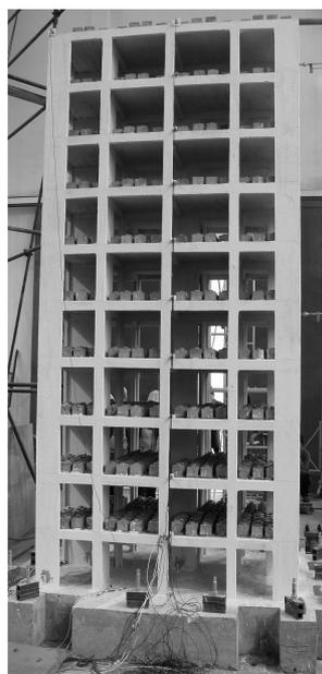
Figure 4 Finished frame-shearwall model
