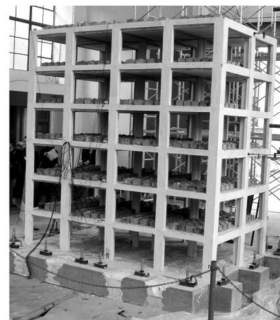
Figure 3 Finished frame model
