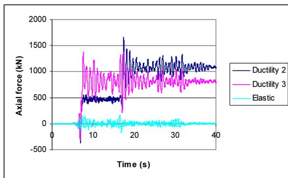
**Figure 6** Variation of transfer forces for different structural ductility levels at level 1 of the structure
