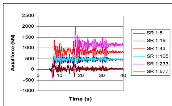
Figure 5 Transfer forces for various frame-wall stiffness ratios at level 1 for 9-storey structure
