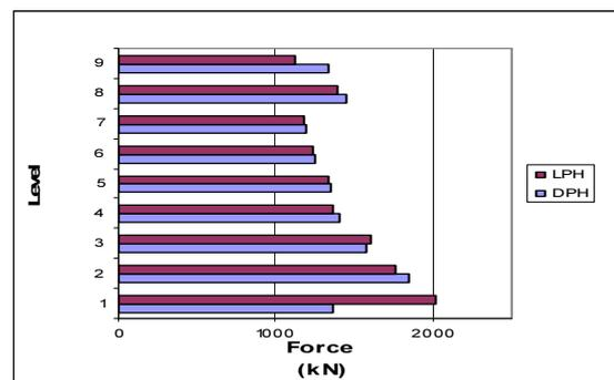
**Figure 11 Comparison between total floor forces for models with lumped and distributed plastic hinge representations**
