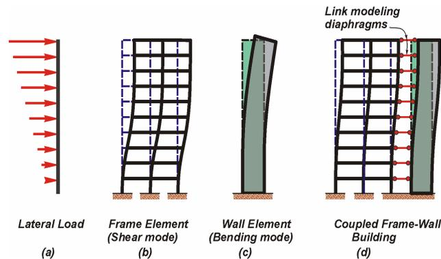
Figure 1 Deformation patterns for frame and wall elements[11]
