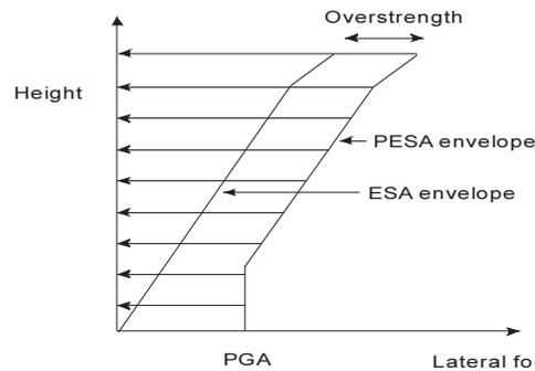
Figure 2 Static forces for ESA and pESA envelopes
