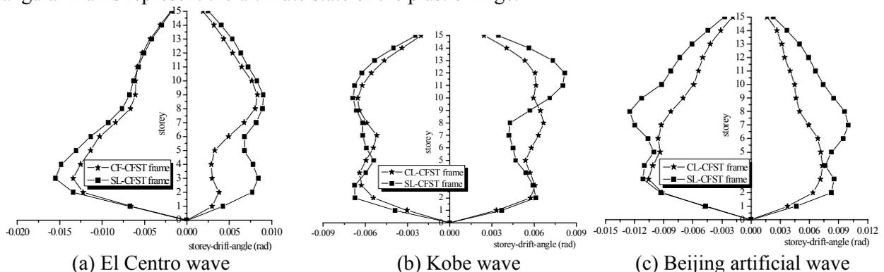
Figure 8 Enveloping values of the storey-drift-angle under the rare earthquake
