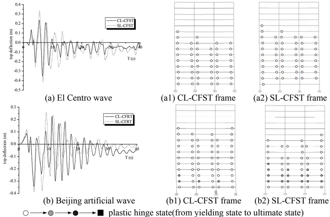
Figure 9 Inelastic displacement time history in Y direction and distribution of plastic hinge
