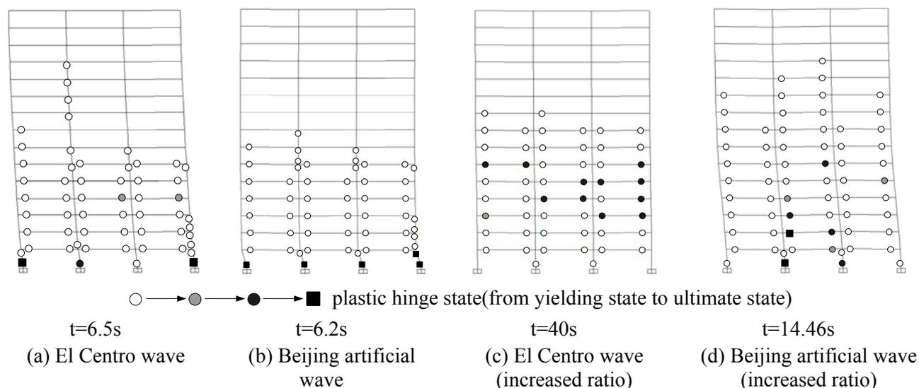
Figure 10 Plastic hinge distribution of the CL-RC column frame
