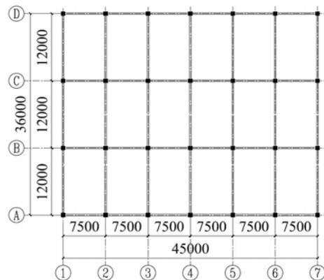
Figure 1 Structural plane layout (unit: mm)
