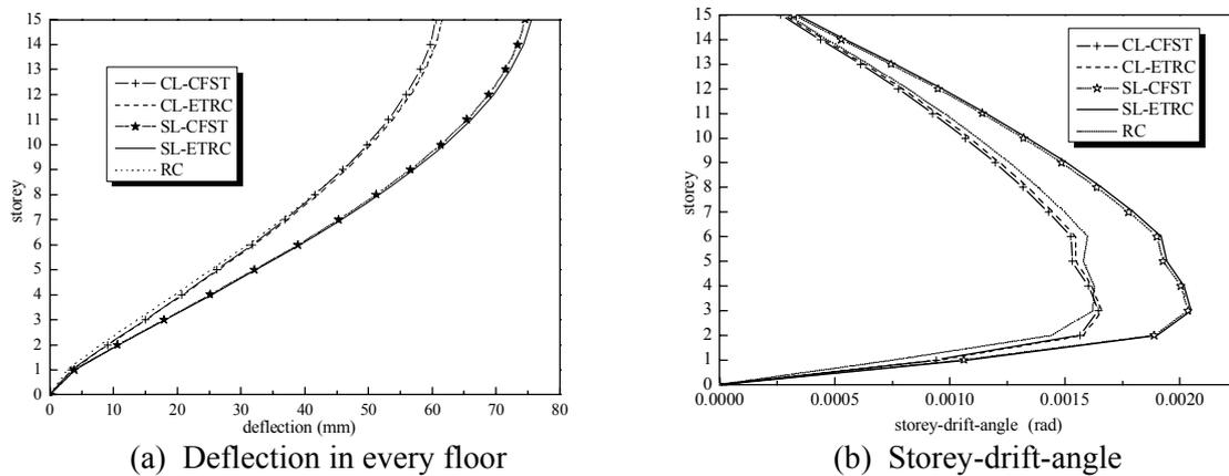
Figure 5 Deflections and storey-drift-angles for frames under earthquake loads in Y direction
