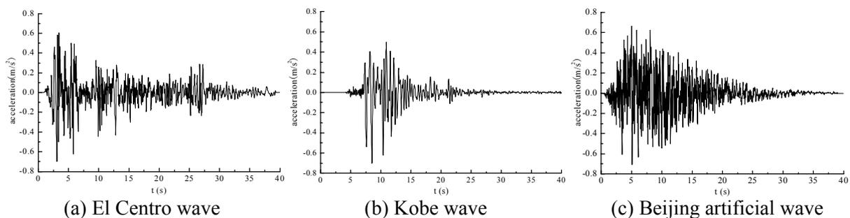
Figure 6 Seismic acceleration time history for elastic time history analysis
