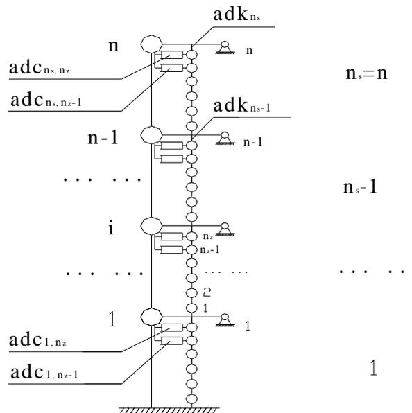
Figure 3 The computing model of the new PMSCS
