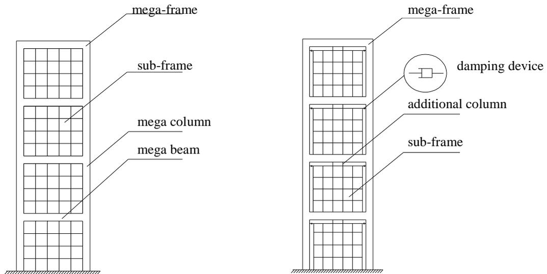
Figure 1 The conventional mega-sub structure
