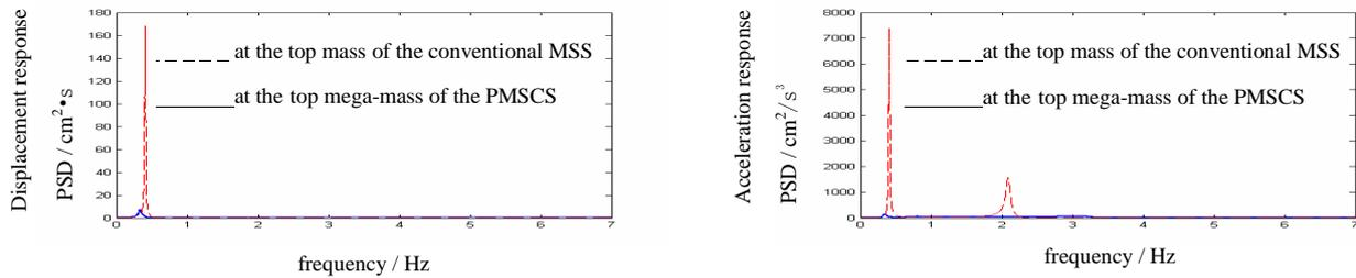
(a) The comparison of the displacement response *PSD*      (b) The comparison of the acceleration response *PSD*
