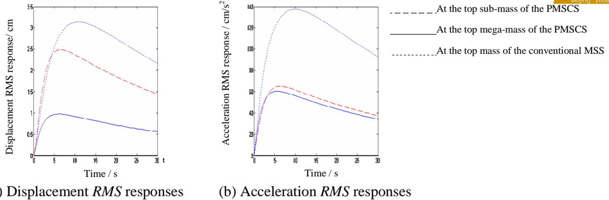
Figure 7 The comparison of *RMS* responses of the two structures, as  $RK=0.17$ , under nonstationary seismic excitation.
