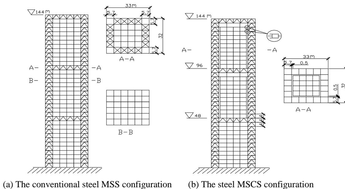
Figure 4 The two structural configurations
