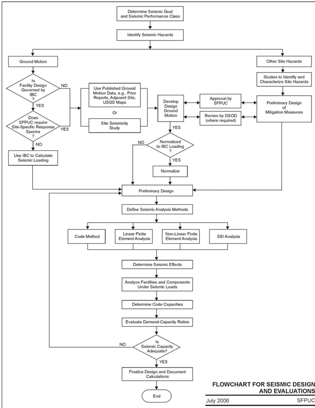
Fig. 2 Flowchart for Seismic Design and Evaluation
