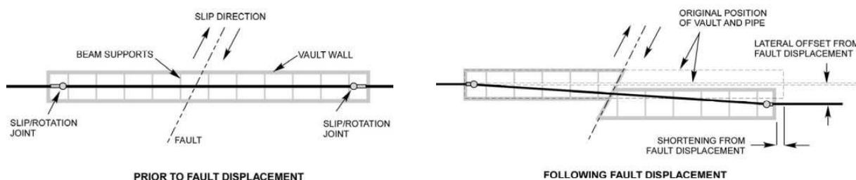
Figure 2. Selected Alternative Fault-Crossing Concept
