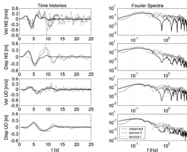
Figure 3 Comparison between NS components of observed (bold line) and simulated velocities and displacements time histories (left) and respective Fourier spectra (right) at the Düzce station. Results obtained in linear behaviour with both the source model I (dotted line) and II (thin line) are shown
