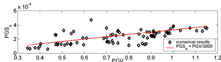
Figure 6 Horizontal  $PGS_a$  vs. PGV obtained by numerical simulations (open symbols) along the NS cross-section and estimated by equation 1.1 ( $PGV / C_{ap.}$ ) with  $C_{ap.}=3000$  (thin line)
