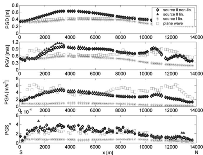
Figure 4 Comparison of surface ground response along the NS cross-section in terms of horizontal peak ground displacement (PGD), velocity (PGV), acceleration (PGA) and longitudinal strain ( $PGS_a$ ). The results have been obtained with the DRM procedure using both the source model I and II, and with a 2D SE analysis using a plane wave as input motion. The origin of the x-axis denotes the Southern basin edge
