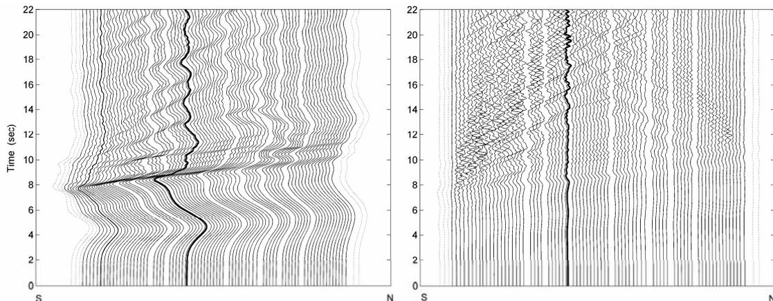
Figure 5 Horizontal displacement (left) and strain (right) time histories at receivers located along the NS cross-section in the Düzce basin. Dotted lines refer to points out of the basin, the thick one refers to the site of the Düzce station. In the figure time histories are spaced with reference to the relative distance between not equispaced receivers; white strips indicate large distance
