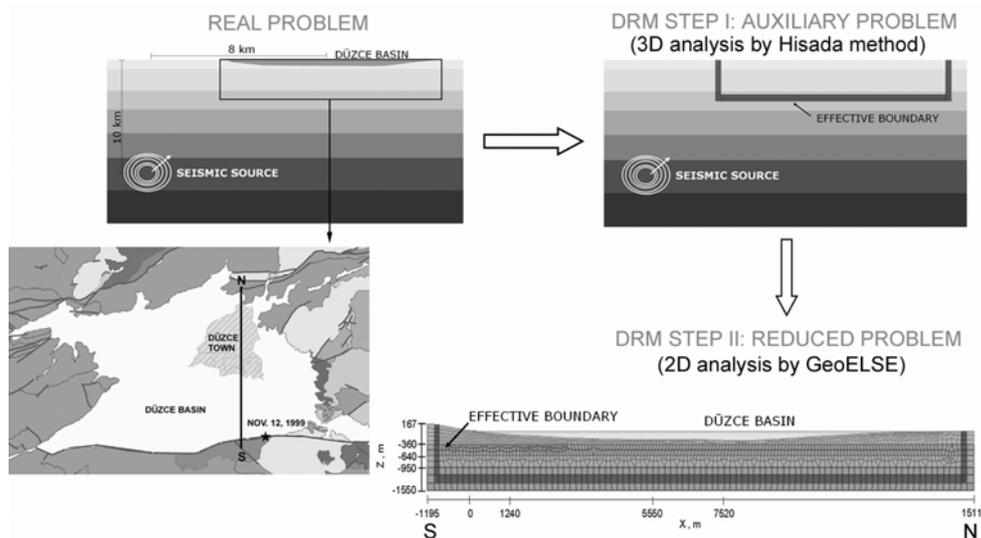
Figure 1 Scheme of the DRM procedure applied to the case of the Düzce urban area. The real problem is subdivided into two simpler ones analyzed in different steps. Step I: 3D analysis of the source and the wave propagation in a layered half-space using the semi-analytical method of Hisada & Bielak (2003). Step II: 2D wave propagation in the Düzce basin, along a NS cross-section, by means of the Spectral Element Method
