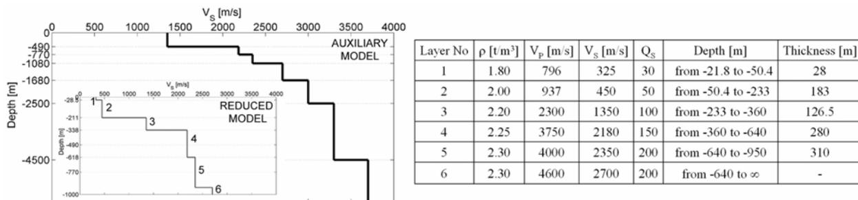
Figure 2 Left:  $V_s$  profile adopted for the first step analyses (bold line): Boore and Joyner, (1997) model for generic rock site (an average value for the uppermost 490 m has been assumed). The profile at the Düzce accelerograph station on the 2D cross-section used in the second step is inserted (thin line). Dynamic soil properties for the reduced model, referring to the Düzce accelerograph station are reported (right).
