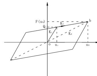
Fig.2: Bilinear hysteretic model of LRB
