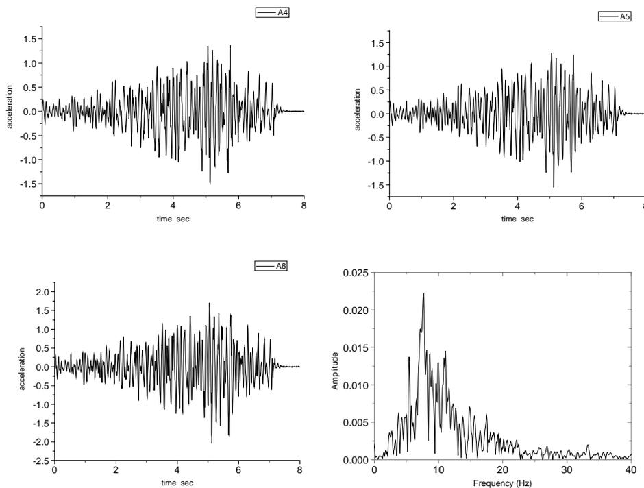
Figure 3. Acceleration time-history and Fourier spectrum of the model subjected to Hujialou record with  $a_{max}=1.0g$  at measurement A4, A5 and A6 as shown in Fig. 1
