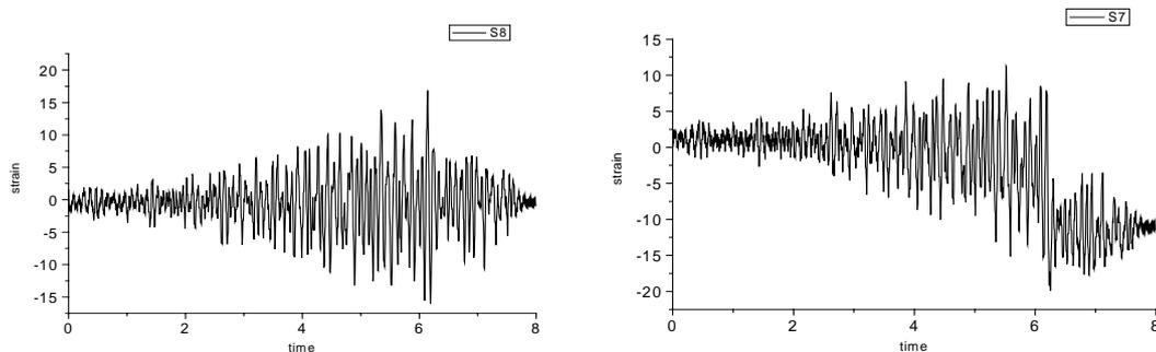
Figure 6. Acceleration time-histories of pipeline and cable inside utility tunnel under excitation of Hujialou record with  $a_{max}=0.6g$
