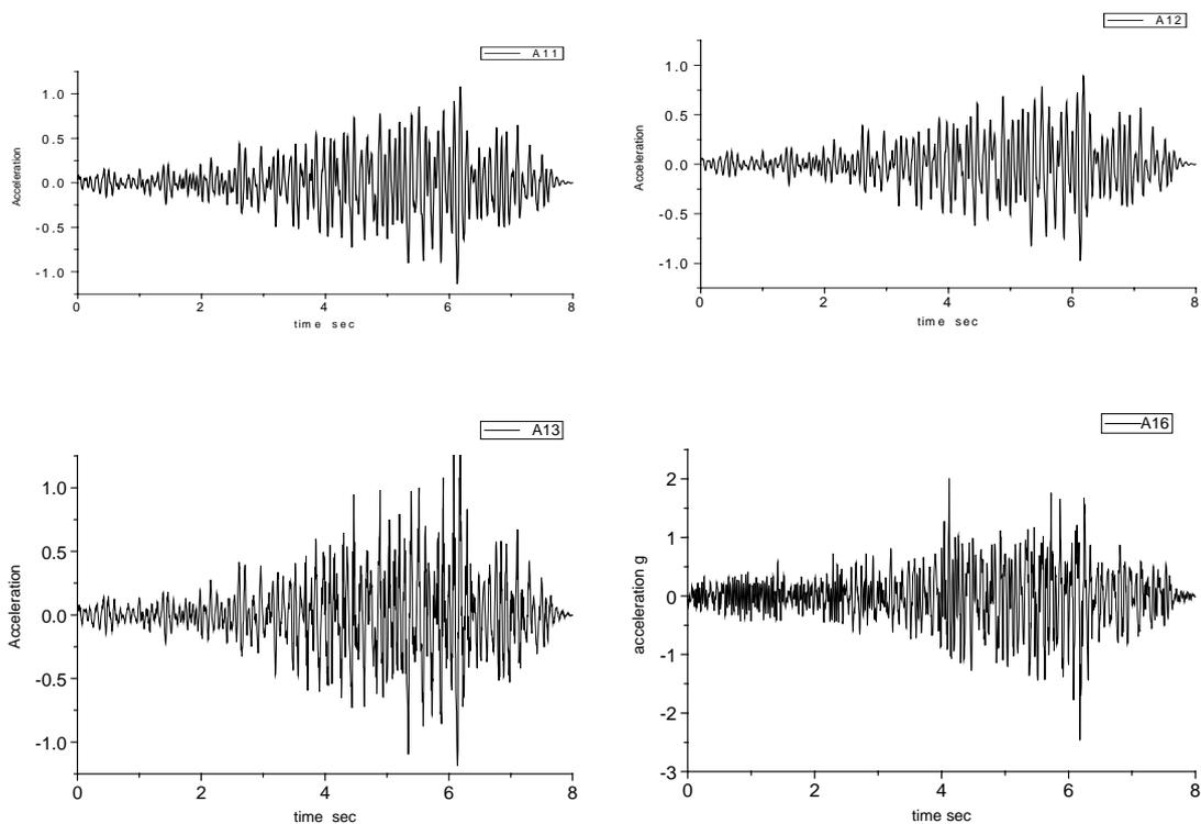
Figure 4. Acceleration time-history of pipeline and cable inside utility tunnel under excitation of Hujialou record with  $a_{max}=0.6g$
