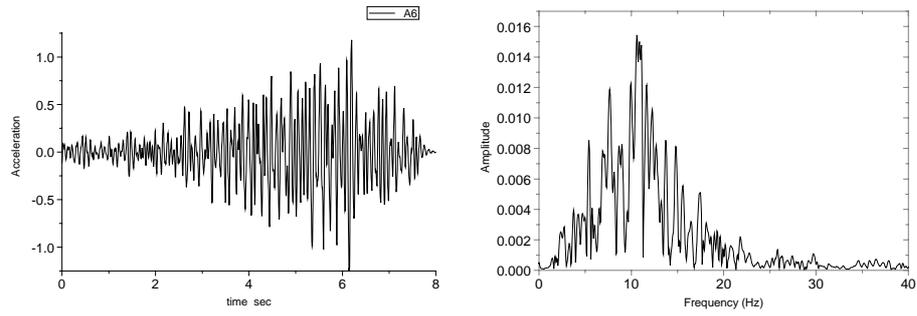
Figure 2. Acceleration time-history and Fourier spectrum (Hujialou record,  $a_{max}=0.6g$ )
