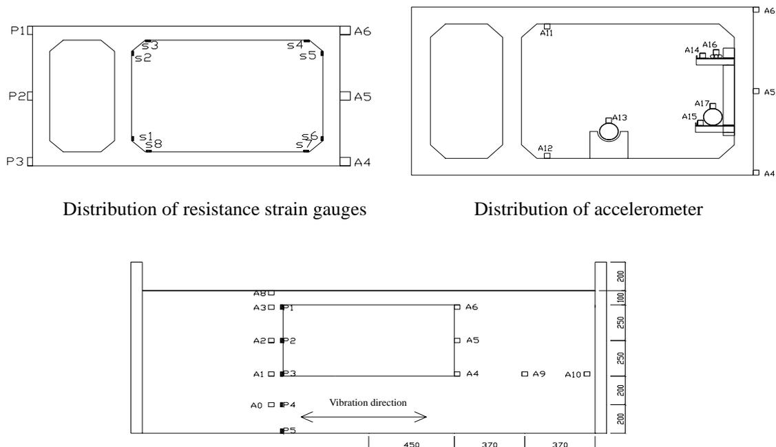
Figure. 1 Distribution of acceleration seismograph and pressure gauge inside soil
