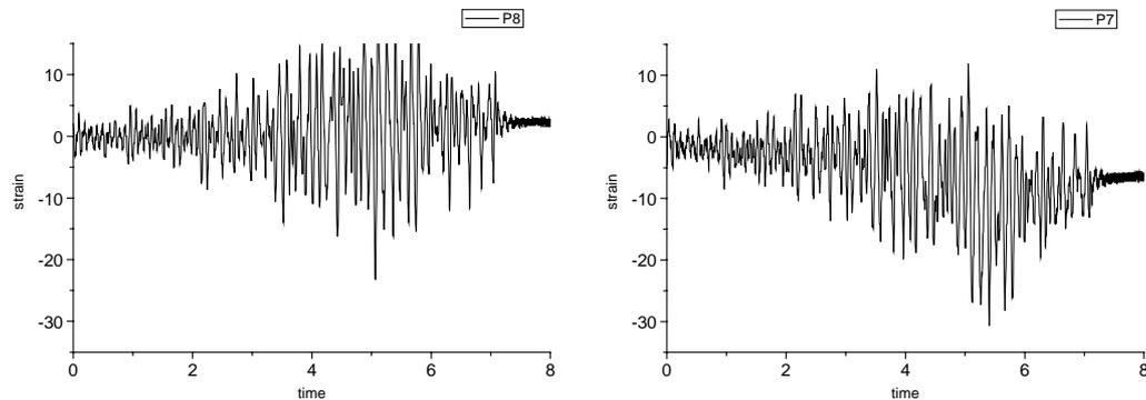
Figure 7. Acceleration time-histories of pipeline and cable inside utility tunnel under excitation of Hujialou record with  $a_{max}=1.0g$
