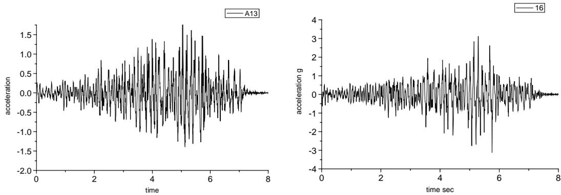
Figure 5. Acceleration time-history of pipeline and cable inside utility tunnel under excitation of Hujialou record with  $a_{max}=1.0g$
