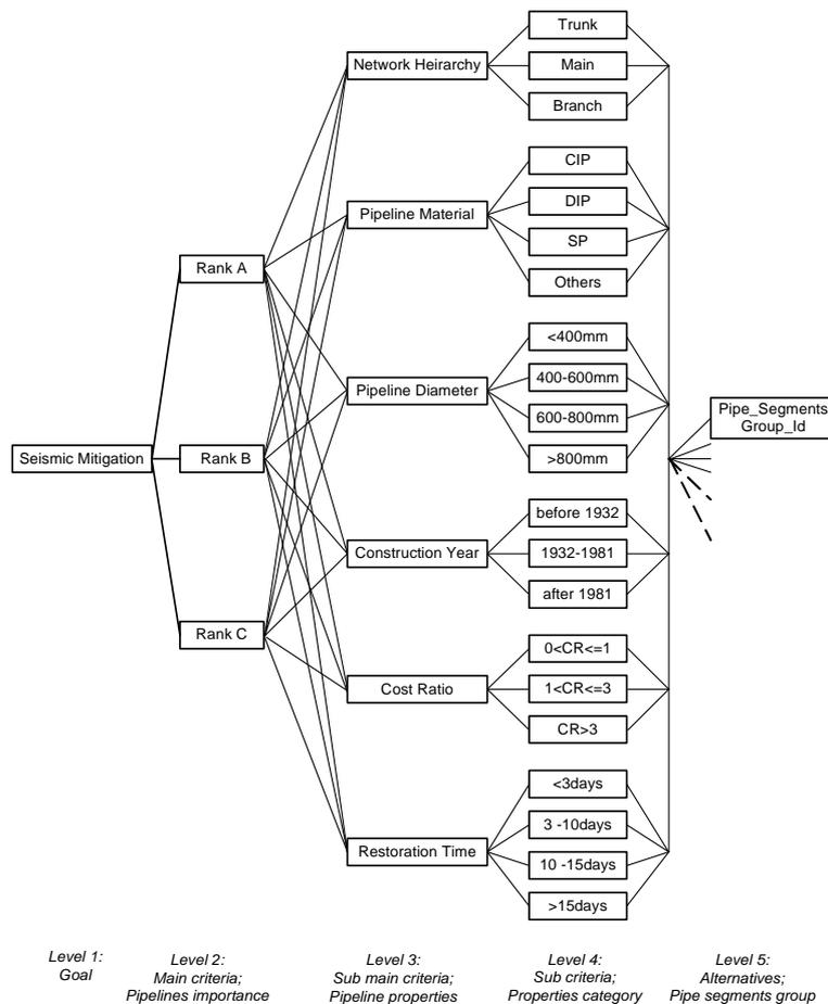
Figure 4 Hierarchy structure of the FAHP prioritization for seismic mitigation of pipeline networks
