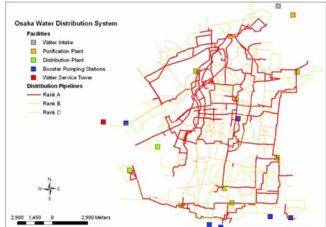
Figure 3 Importance rank assignment to pipelines
