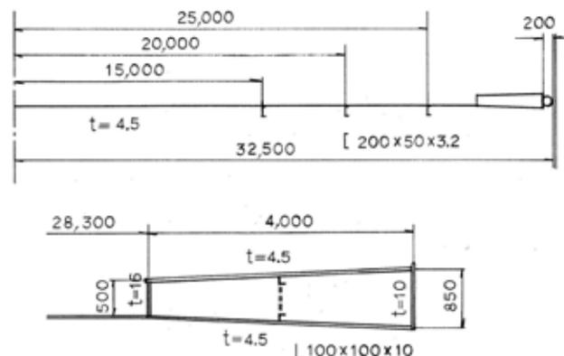
Figure 1 Analyzed model of single-deck floating-roof
