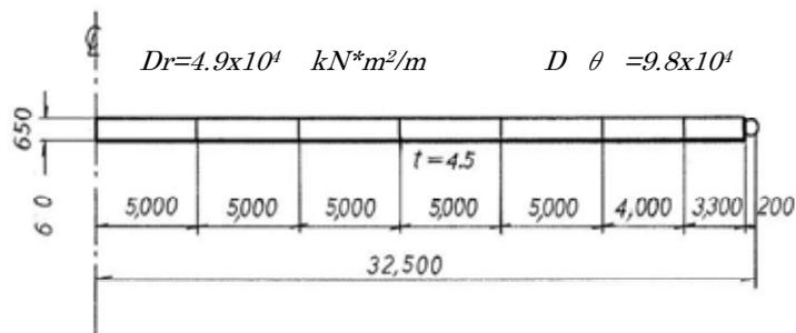
Figure 2 Analyzed model of double-deck floating-roof
