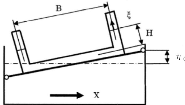
Figure 5 TLCD set on floating-roof of oil tank
