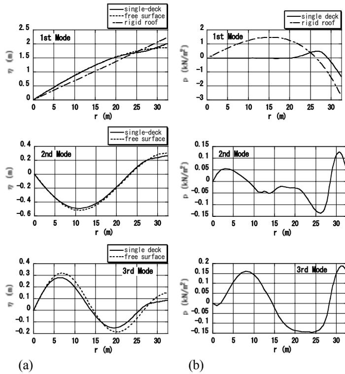
Figure 3 Modal response in the case of single-deck floating-roof: (a) displacement, (b) dynamic pressure
