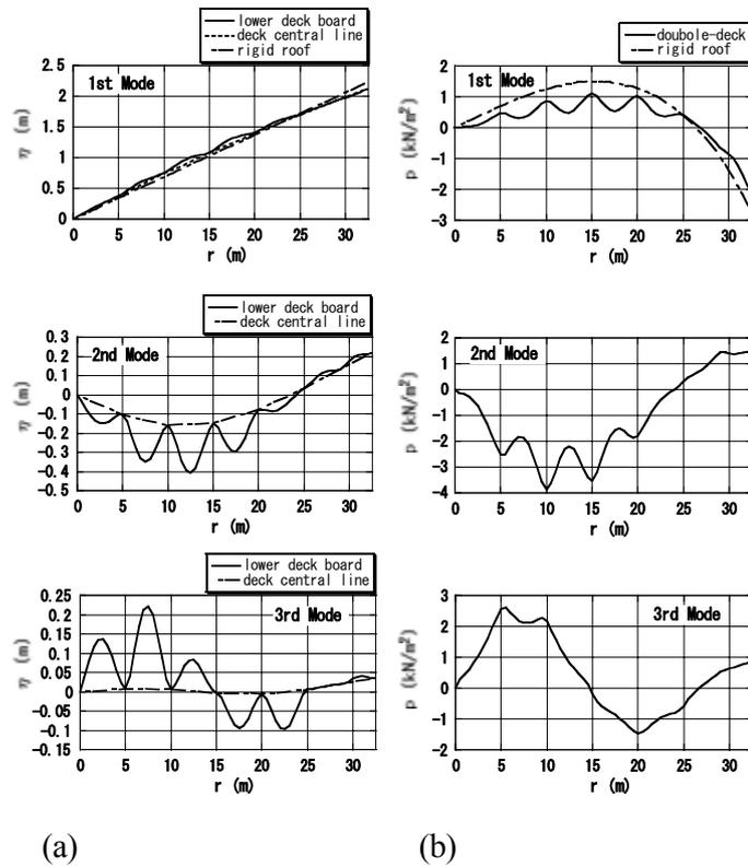
Figure 4 Modal response in the case of double-deck floating-roof: (a) displacement, (b) dynamic pressure
