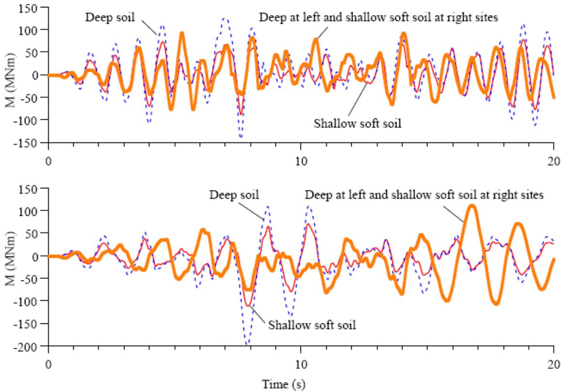
Figure 5. Influence of local soil conditions on bending moment development at bridge pier supports
