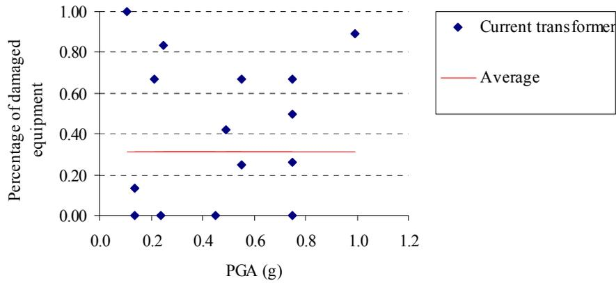
Figure 9 Percentage of damaged current transformers in medium- and high-voltage substations
