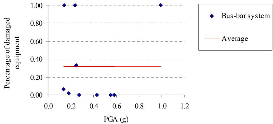
Figure 11 Percentage of damaged bus-bar systems in medium- and high-voltage substations
