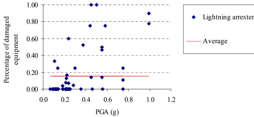
Figure 12 Percentage of damaged lightning arresters in medium- and high-voltage substations
