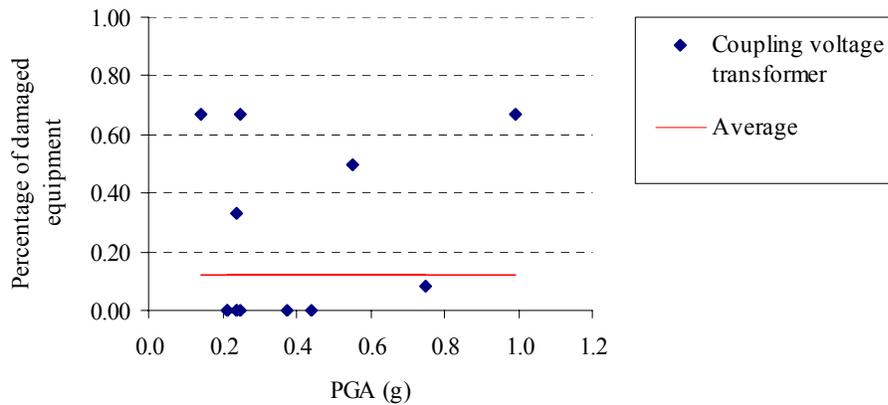
Figure 14 Percentage of damaged capacitive coupling voltage transformer in medium- and high-voltage substations
