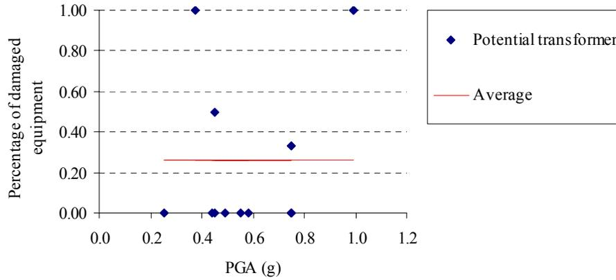
Figure 10 Percentage of damaged potential transformers in medium- and high-voltage substations
