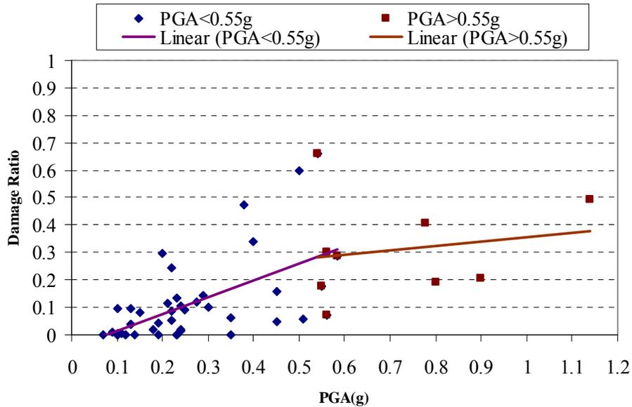
Figure 15 Damage ratio curve of the medium and high voltage substations
