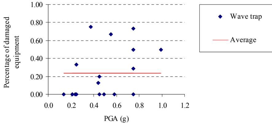
Figure 13 Percentage of damaged wave traps in medium- and high-voltage substations
