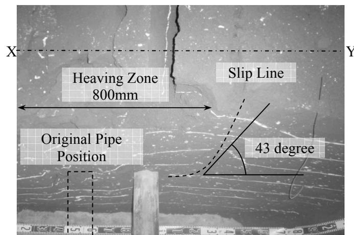
Figure 4 Ground deformation after Test 2 (dense backfill conditions)
