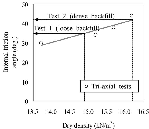
Figure 3 Relationship between dry weight and internal friction angle
