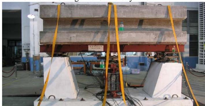
Figure2 The 1/10 isolated bridge model
