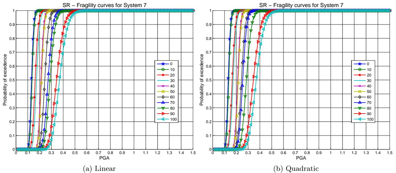
Figure 5: Service Reduction, SR: Linear and Quadratic Capacity
