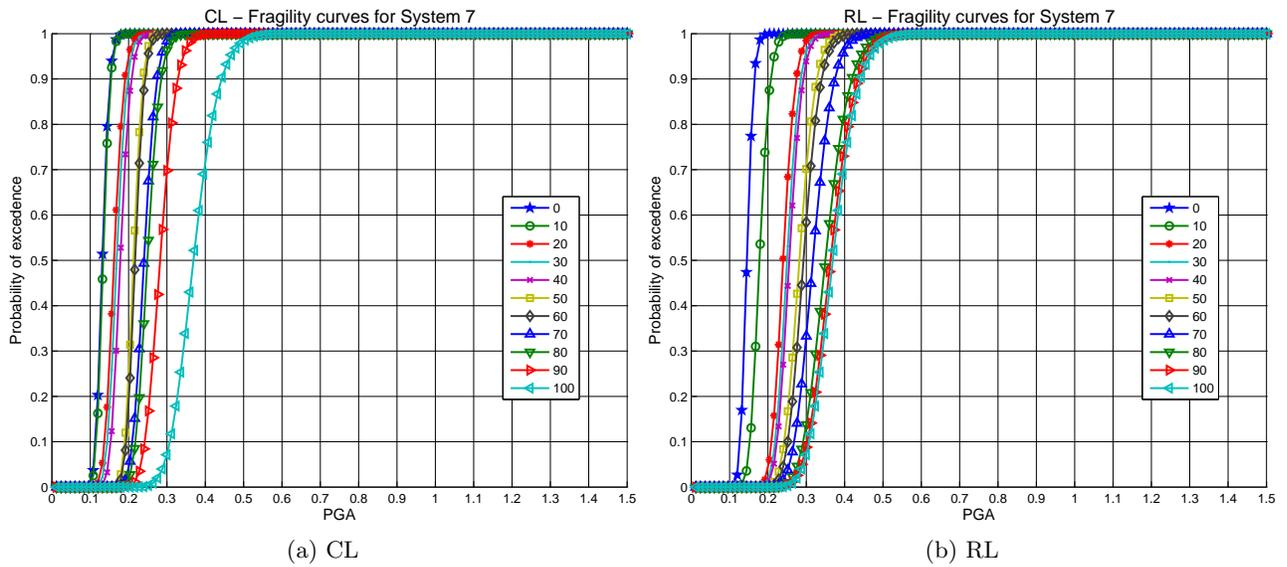
Figure 4: Connectivity (CL) and Reachability Loss (RL)
