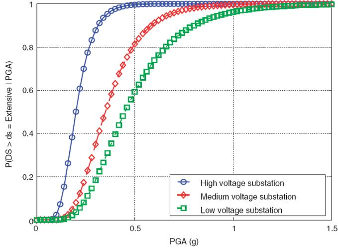
Figure 3: Fragility curves for network's nodes
