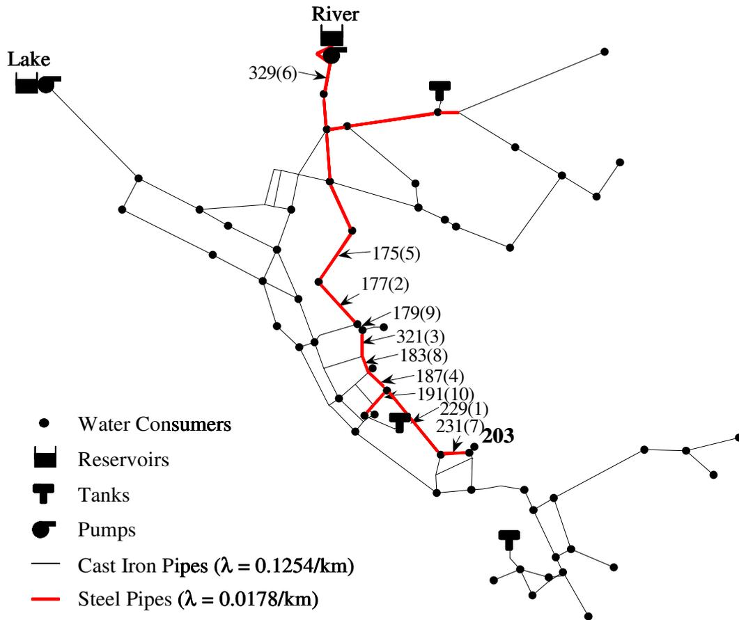
Figure 3. Spatial Distribution of Critical Links from UBI Efficient Frontier for Node 203 (Number in the parenthesis after the pipe ID indicates the order of adding the critical links to the critical link group)
