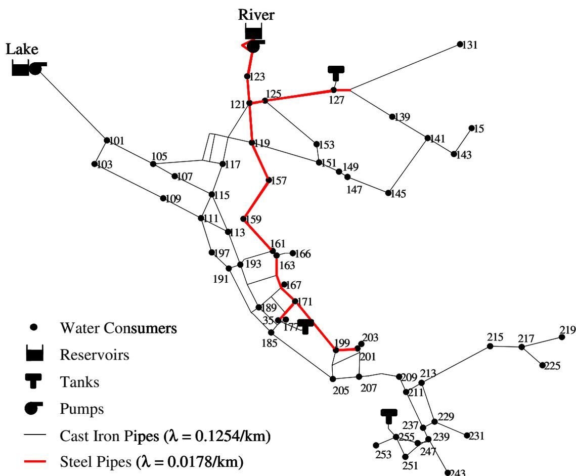
Figure 1. Schematic View of a Hypothetical Water Supply System
