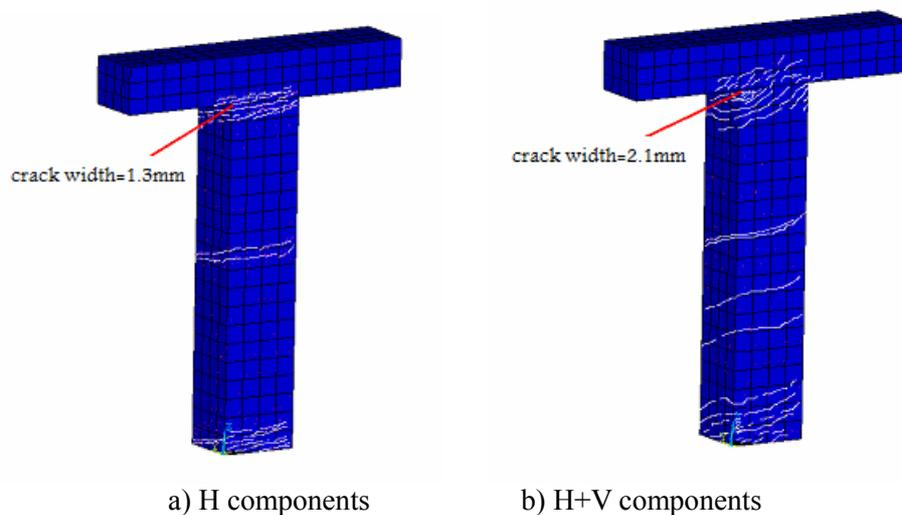
Figure 9 Crack pattern of model A subjected to a) H components and b) H+V components of Tabas record with PGA=0.5g.
