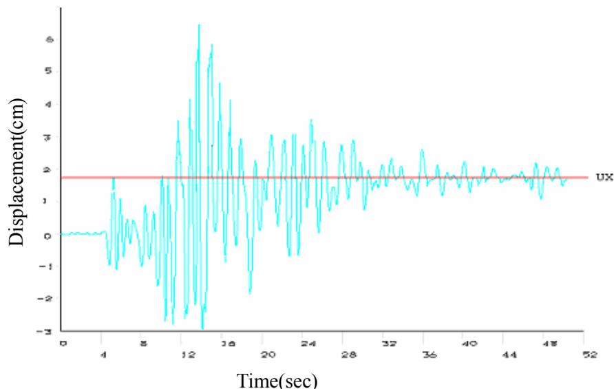
Figure 8 Deck lateral displacement time history of model A subjected to H+V component of Tabas record with PGA=0.3g.
