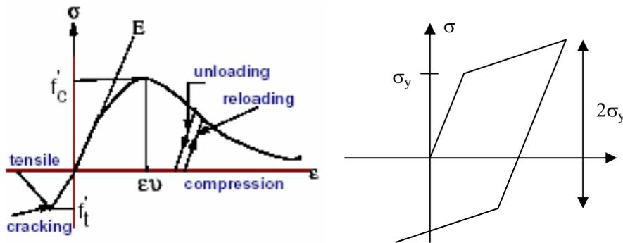
a) Concrete      b) Steel reinforcement
