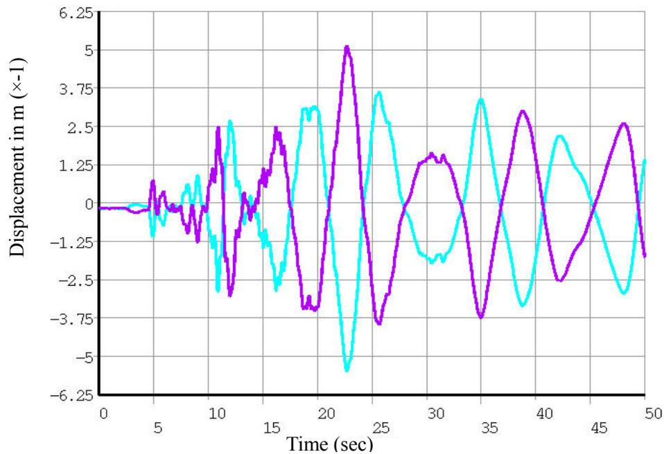
Figure 4 Sloshing displacements time history of tank type 22 due to Tabas record
