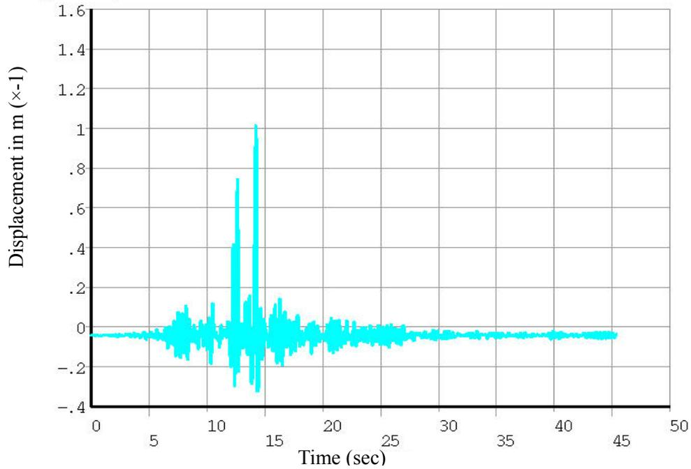
Figure 3 Uplift displacement time history of tank type 22 due to Tabas record
