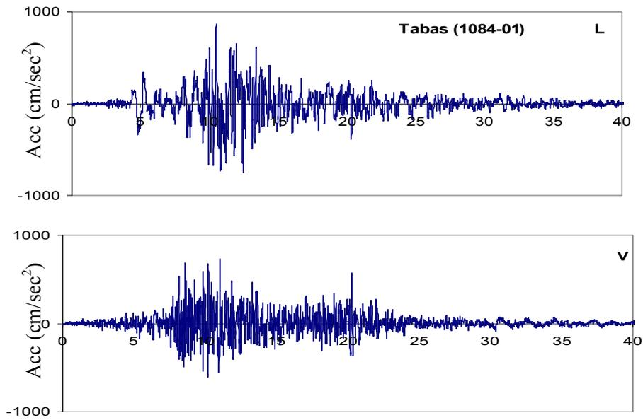
Figure 2 Horizontal (L) and vertical (V) component Tabas record
