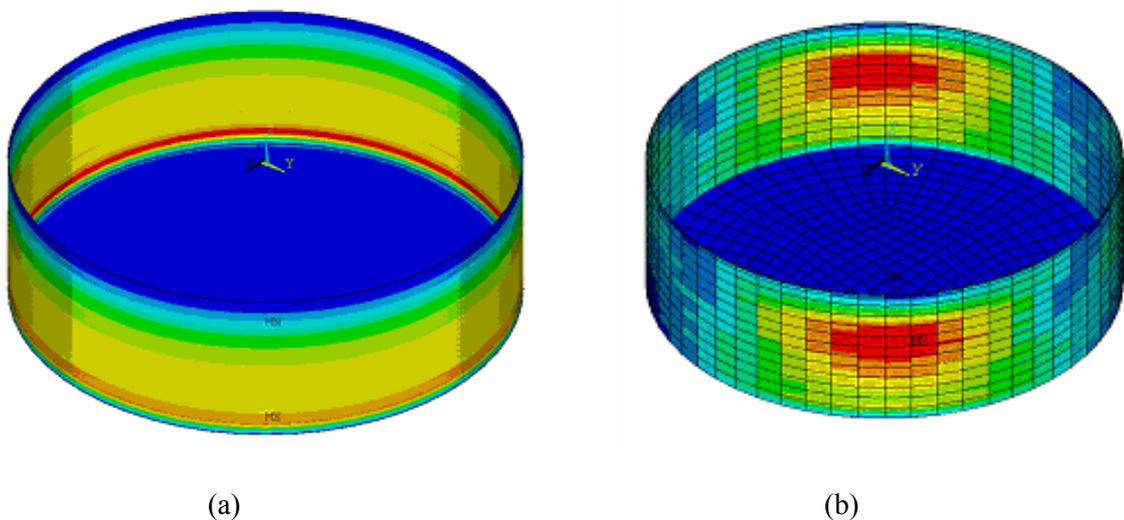
Figure 2 Von-misses stresses of tank shell due to a) hydrostatic forces and b) spectral forces
