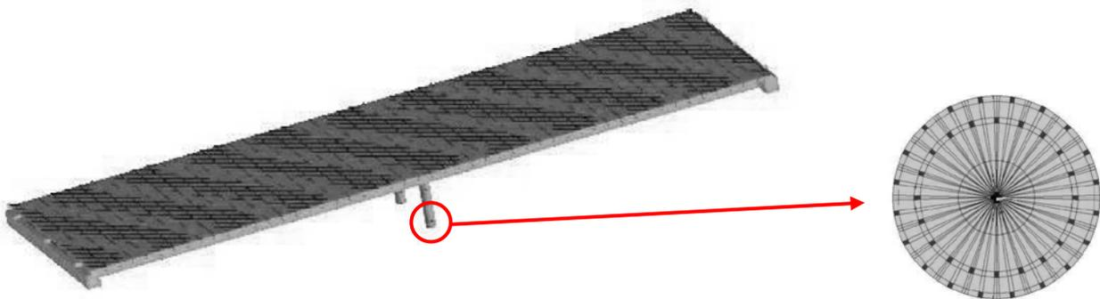
Figure 1 FEM Model of 12.3° skew bridge (l.) and modeled reinforced concrete column cross section (r.)
