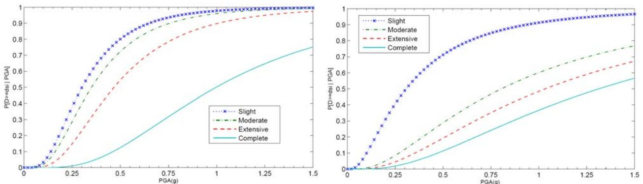
Figure 7 Fragility curve of column for no-skew (l.), Fragility curve of bearing for no-skew (r.)
