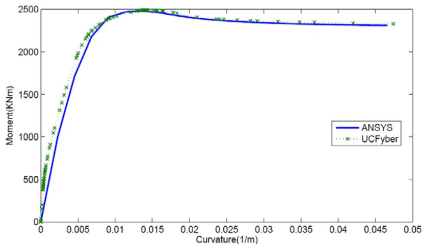
Figure 3 Moment-Curvature relationship comparison
