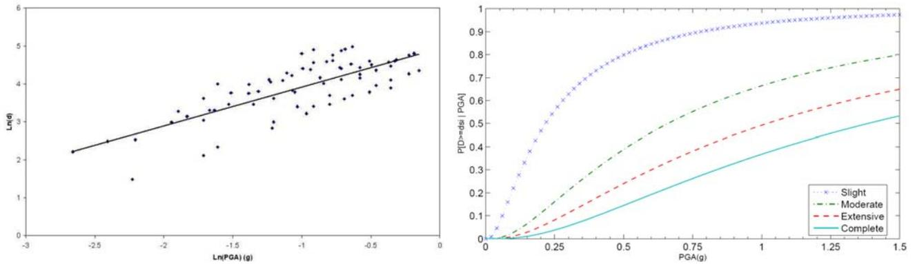
Figure 6 Linear regression of bearing for 12.33° skew bridge (l.), Fragility curve of bearing for 12.33° skew (r.)
