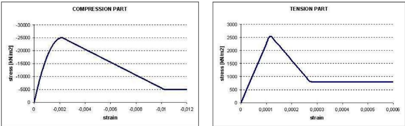
Figure 2 Concrete material model for compression and tension
