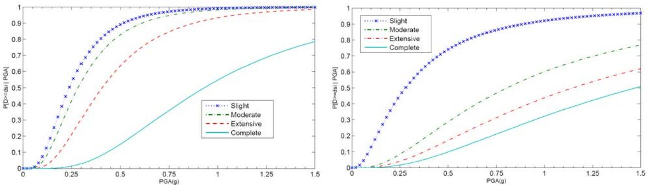
Figure 8 Fragility curve of column for 45° skew (l.), Fragility curve of bearing for 45° skew (r.)
