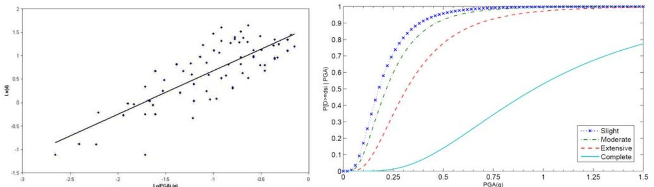
Figure 5 Linear regression of column for 12.33° skew bridge (l.), Fragility curve of column for 12.33° skew (r.)
