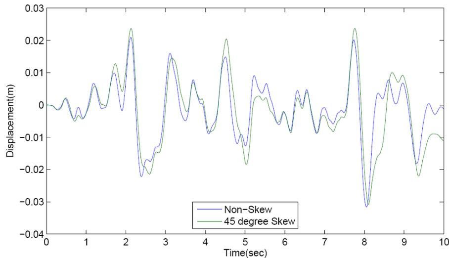
Figure 4 Colum response time history comparison for non-skew and 45° skew bridge
