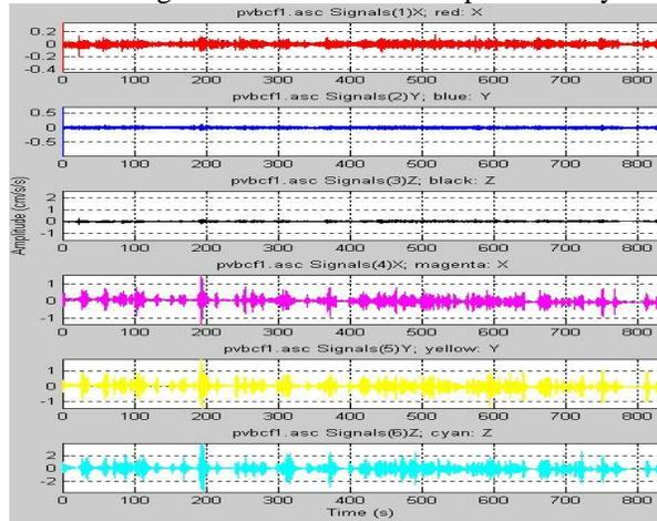
Figure 4 Accelerations measured in two sensors with 3 channels ( $x = \text{longitudinal}$ ,  $y = \text{transversal}$  and  $z = \text{vertical}$ ) in up to down order. Upper signals belong to free field and the bottom ones to deck of Villabonita bridge.
