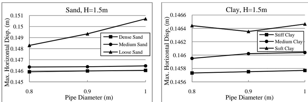
**Figure 7- Effect of Pipe Diameter on Response of Middle Element in Horizontal Direction**
