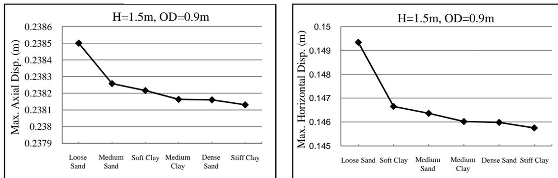
Figure 3- Effect of Soil Stiffness on Response of Middle Element
