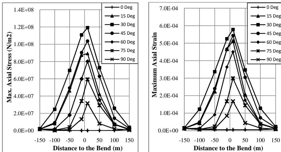
**Figure 12- Maximum Axial Stress & Strain for Models with Different Bend Angles**
