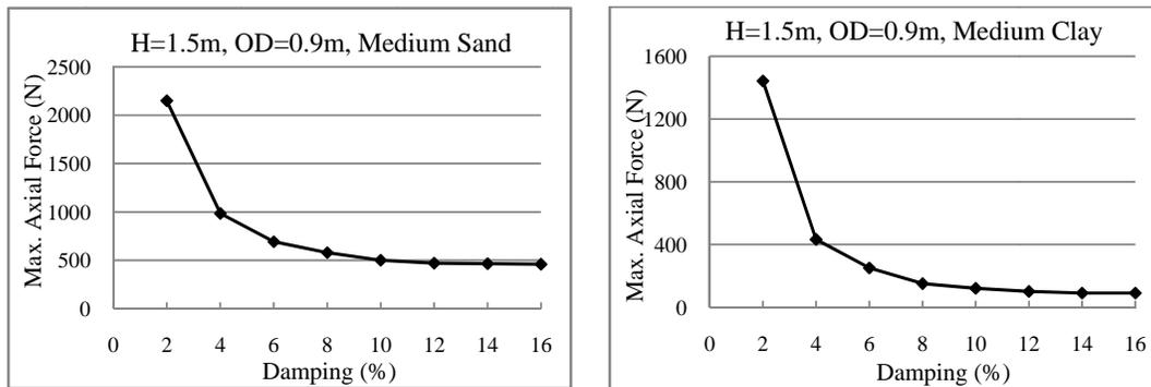
Figure 9- Effect of Soil Damping on Response of Middle Element in Axial Direction
