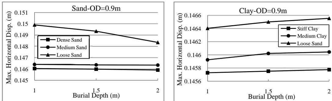
**Figure 5- Effect of Burial Depth on Response of Middle Element in horizontal Direction**
