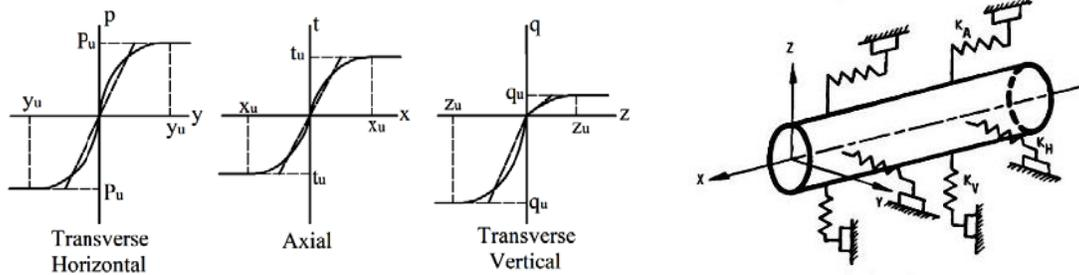
Figure 1- Soil-Pipe Interaction Modeling [7]
