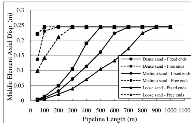
Figure 2- Effect of Boundary Conditions on Maximum Response of Middle Element
