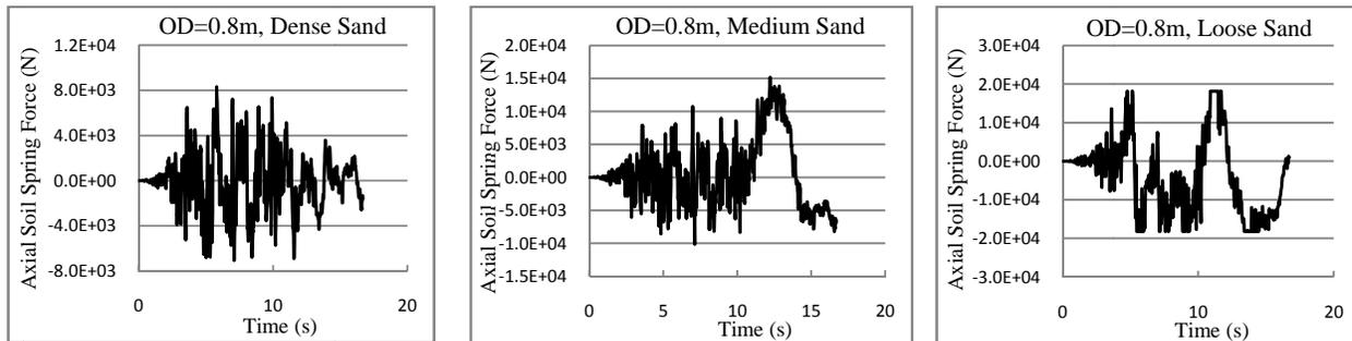
Figure 10- Effect of Soil Damping on Response of Middle Element in Axial Direction
