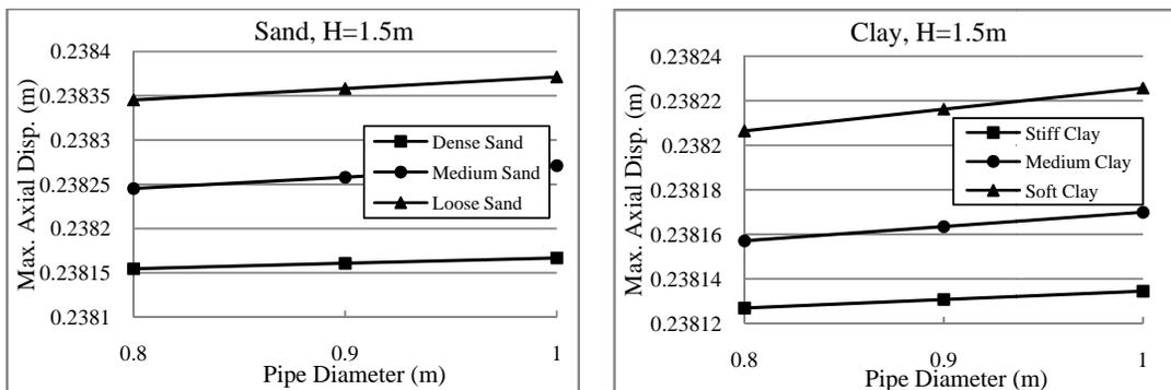
**Figure 8- Effect of Pipe Diameter on Response of Middle Element in Axial Direction**
