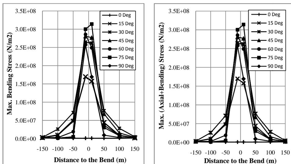
**Figure 13- Maximum Axial Stress for Models with Different Bend Angles**
