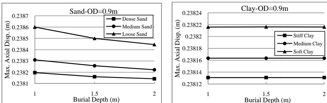
**Figure 6- Effect of Burial Depth on Response of Middle Element in Axial Direction**
