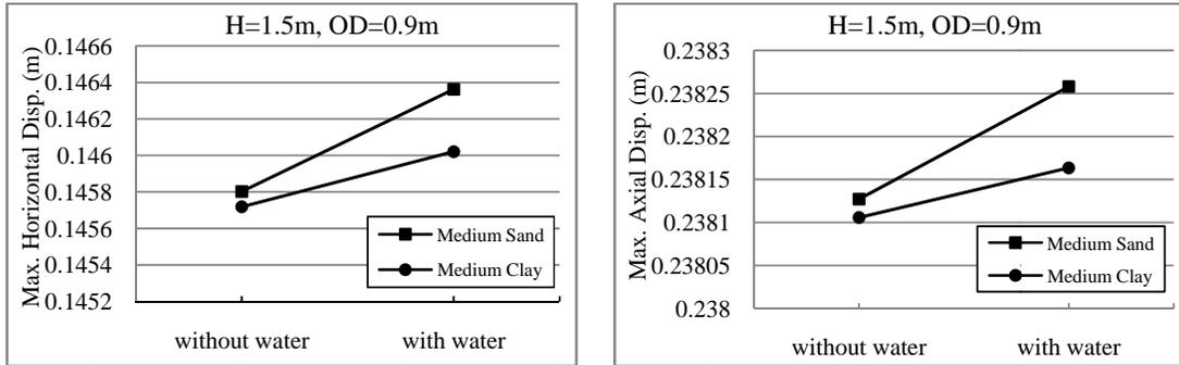
**Figure 4- Effect of Existence of Water on Response of Middle Element**
