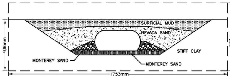
Figure 2.1 Schematic of the cross-section of the 1<sup>st</sup> centrifuge model.
