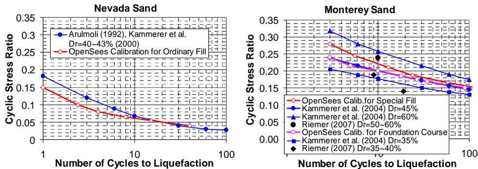
Figure 3.1 Liquefaction resistance calibration of PDMY01 material for the 1<sup>st</sup> centrifuge test.
