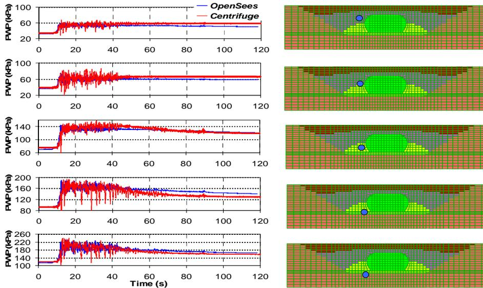
Figure 4.4 Pore water pressures in a vertical column during TCU078 motion for the 1<sup>st</sup> centrifuge test.
