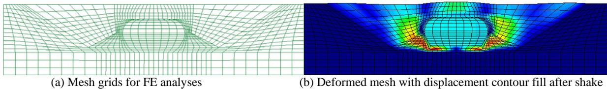
Figure 4.1 FE meshes for the 1<sup>st</sup> centrifuge test.
