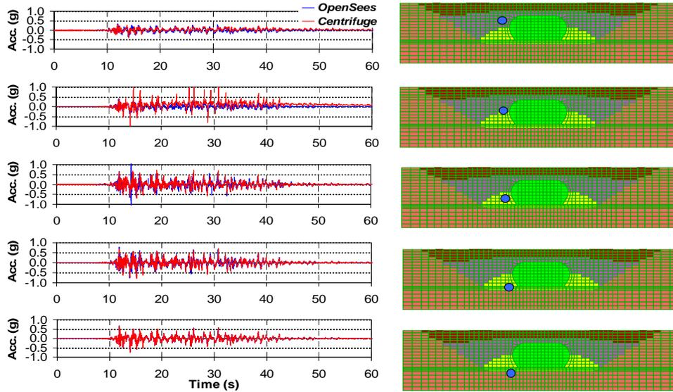
Figure 4.3 Accelerations in a vertical column during TCU078 motion for the 1<sup>st</sup> centrifuge test.
