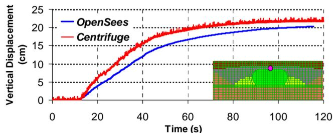
Figure 4.2 Computed and recorded tube uplift during TCU078 motion for the 1<sup>st</sup> centrifuge test.
