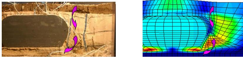
Figure 4.5 Comparison between observed and computed soil deformation pattern.
