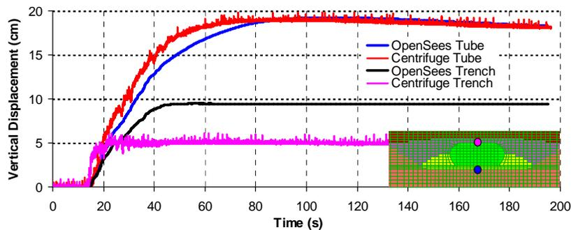
Figure 4.6 Computed and recorded tube and trench uplifts during TCU078 motion for the 2<sup>nd</sup> centrifuge test.
