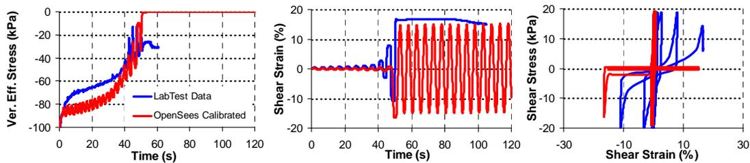
Figure 3.2 Single element dynamic behavior for PDMY01 model calibration (CSR=0.19).
