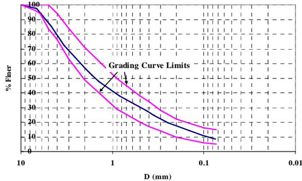
Figure 2 Grain size distribution of tested backfill soil along with specified limits
