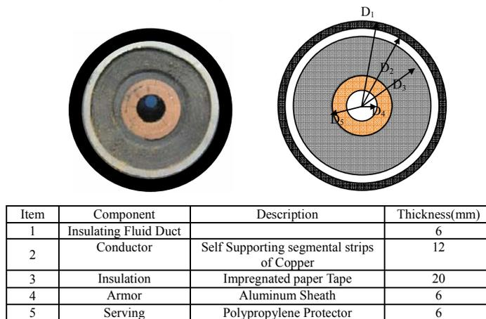
Figure 3 Power Transmission Cable Cross Section
