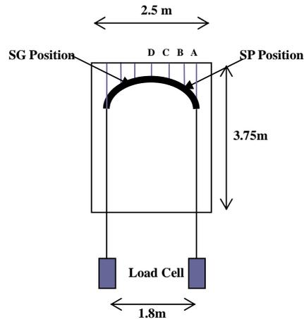
Figure 1 Photograph and schematic diagram showing typical test set up for: (a) axial pullout testing; and (b) lateral pullout testing (SP= String Potentiometer, SG=Strain Gauge)
