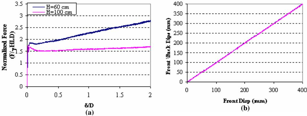
Figure 4 (a) Response of buried cable to axial pullout (Burial depths of 60 and 100 cm)
