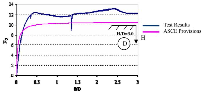
Figure 5 Response of buried cable to lateral pullout (Burial depth of 30 cm). The predicted response using ASCE (1984) equations for buried pipelines is also shown.
