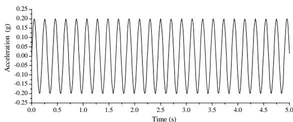
Figure 3 Acceleration time history of 5 Hz sine wave
