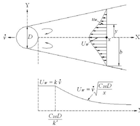
Figure 6 Wake flow for a pipe moving with constant speed in still water
