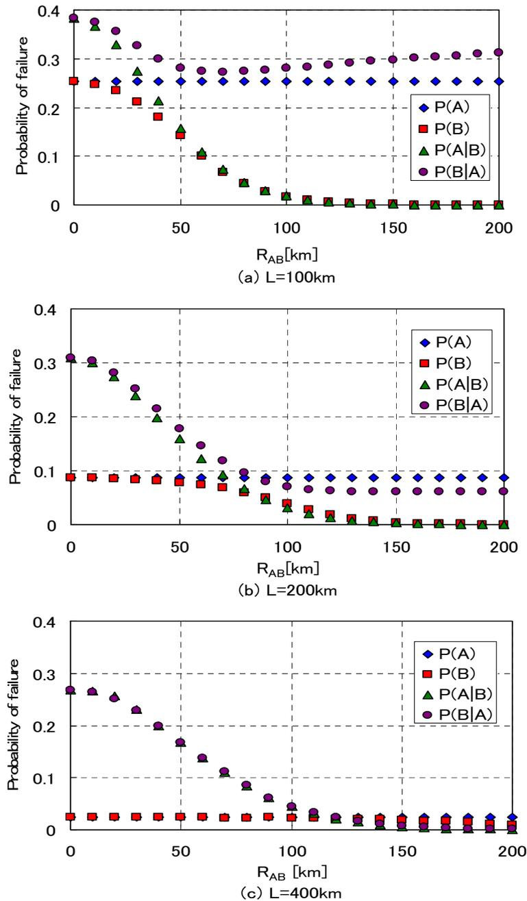
Fig.4 Evaluated probability of failure dependent of the distance between A and B
