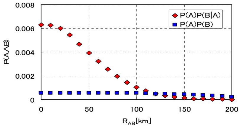
Fig.5 Probability of simultaneous failure for A and B
