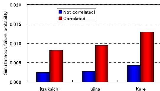
Fig.9 Probability of simultaneous failure for Hatsukaichi and other quay walls
