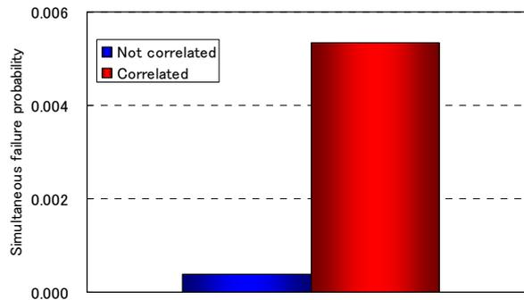
Fig.10 Simultaneous failure probability of whole quay walls with and without considering the correlation
