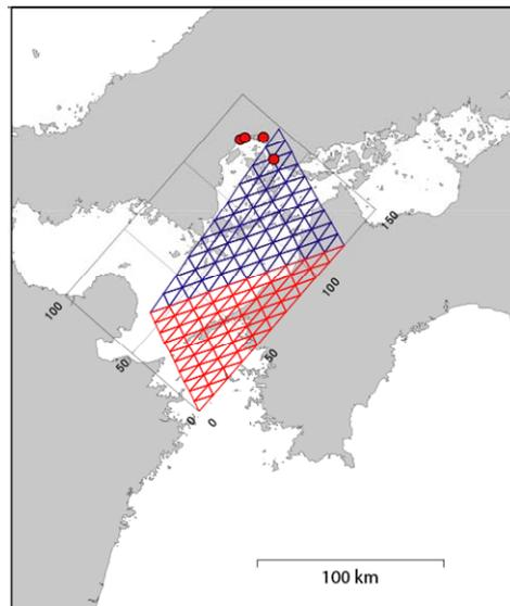
Fig.6 Meshes of possible earthquake source location on the fault
