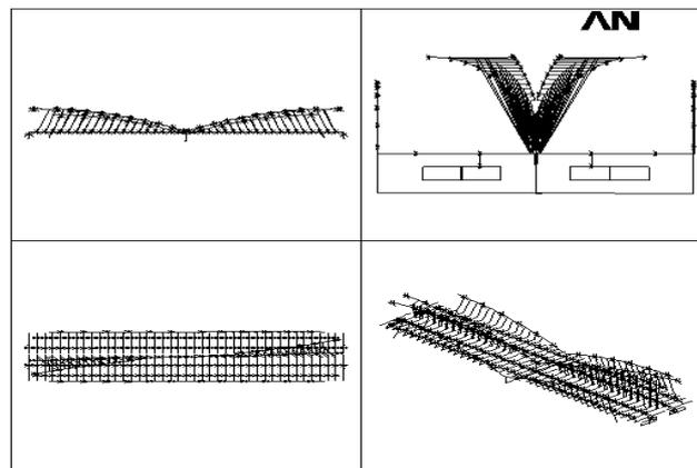
Fig.5 First vibration mode of bridge
