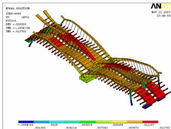
Fig.7 Bridge displacement along bridge axis
