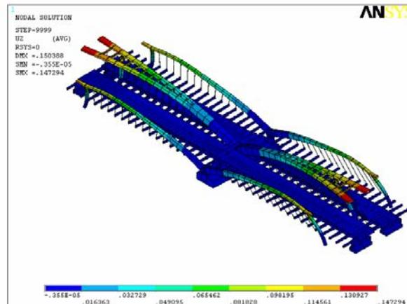
Fig.8 Bridge displacement across bridge axis
