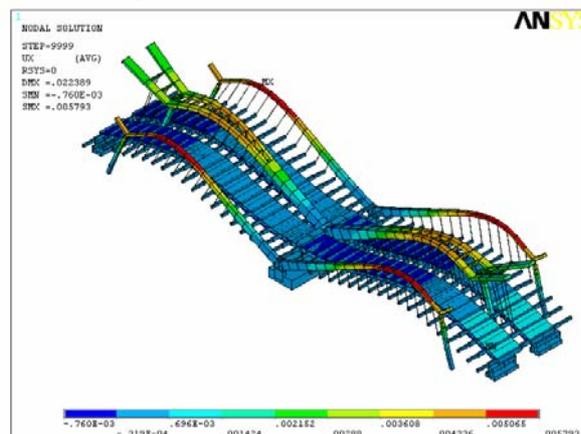
Fig.9 Displacement response in vertical direction
