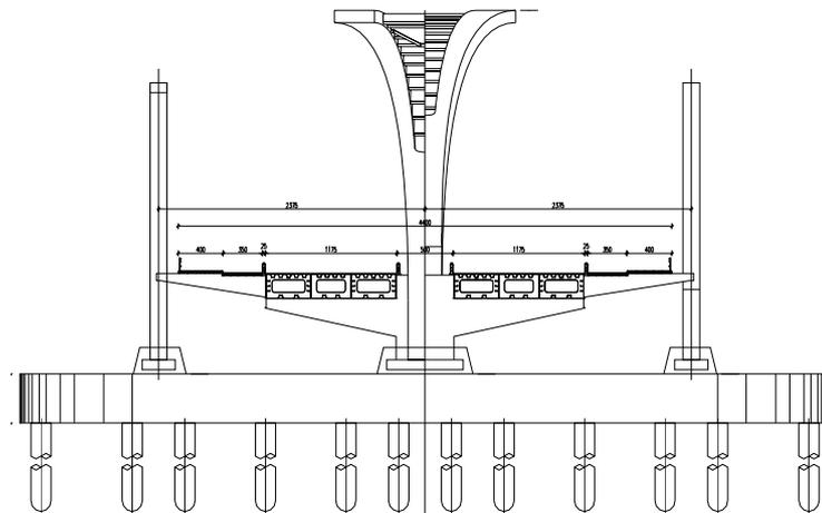
Fig.3 Cross section design of bridge
