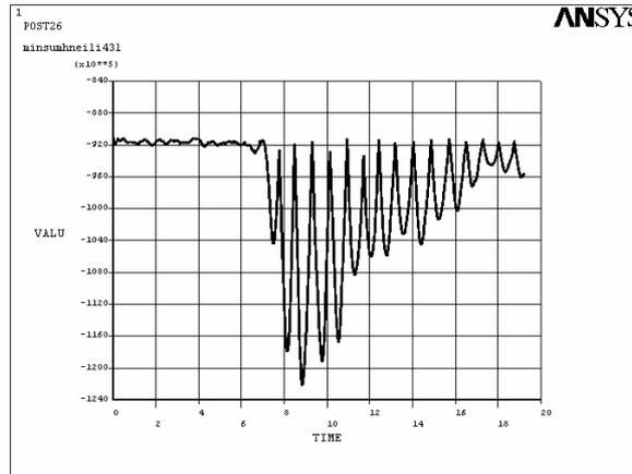
Fig.13 Maximum stress time history of main girder at its bottom(unit: Pa)
