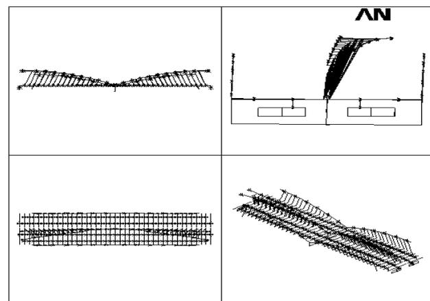
Fig.6 Second vibration mode of bridge
