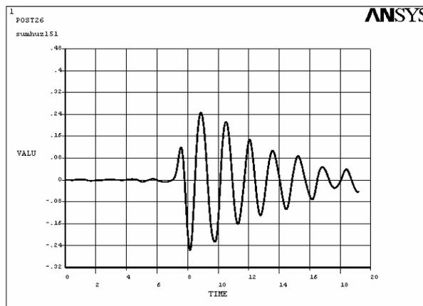
Fig.14 Displacement time history of main wing at tip in lateral direction (unit: m)
