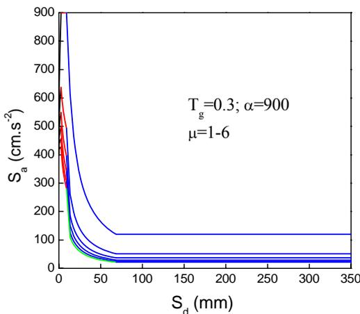
(a) The demand spectra under 8 degree Infrequency Earthquake of I site condition
