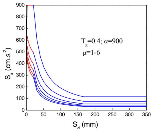
(b) the demand spectra under 8 degree Infrequency Earthquake of II site condition
