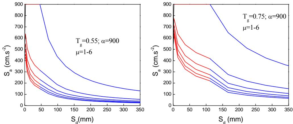
(c) The demand spectra under 8 degree Infrequency Earthquake of III site condition
