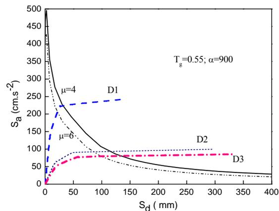
Figure 5 The PUSH-OVER analysis result of example structures
