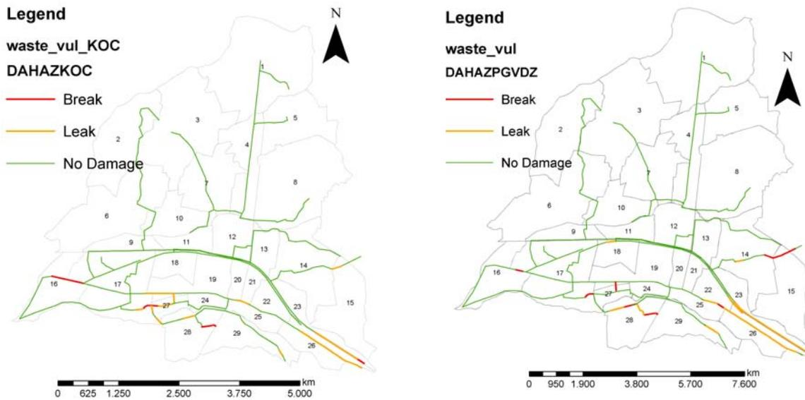
Figure 7 Spatial distribution waste-water pipe damages for Kocaeli (left) and Düzce (right) earthquake
