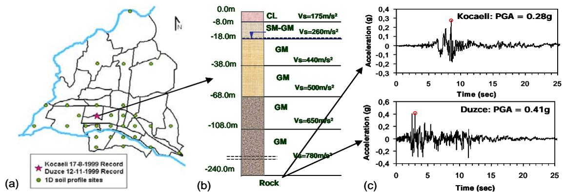
Figure 3 (a) Location of 1D site response analyses, (b) Vs (m/sec) profile at the Meteorological Station and (c) deconvoluted time histories of Kocaeli and Düzce earthquakes, used as input motions for the 1D EQL analyses
