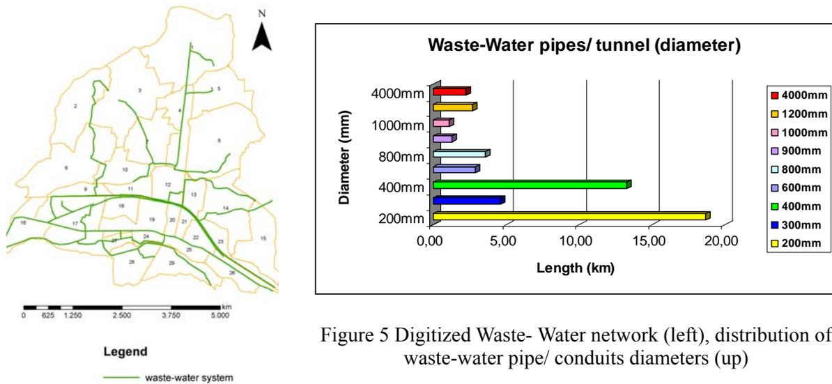
Figure 5 Digitized Waste- Water network (left), distribution of waste-water pipe/ conduits diameters (up)
