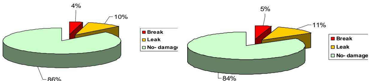
Figure 6 Estimated damages of waste-water network as percentage of the total length of the network for Kocaeli (left) and Düzce (right) earthquake
