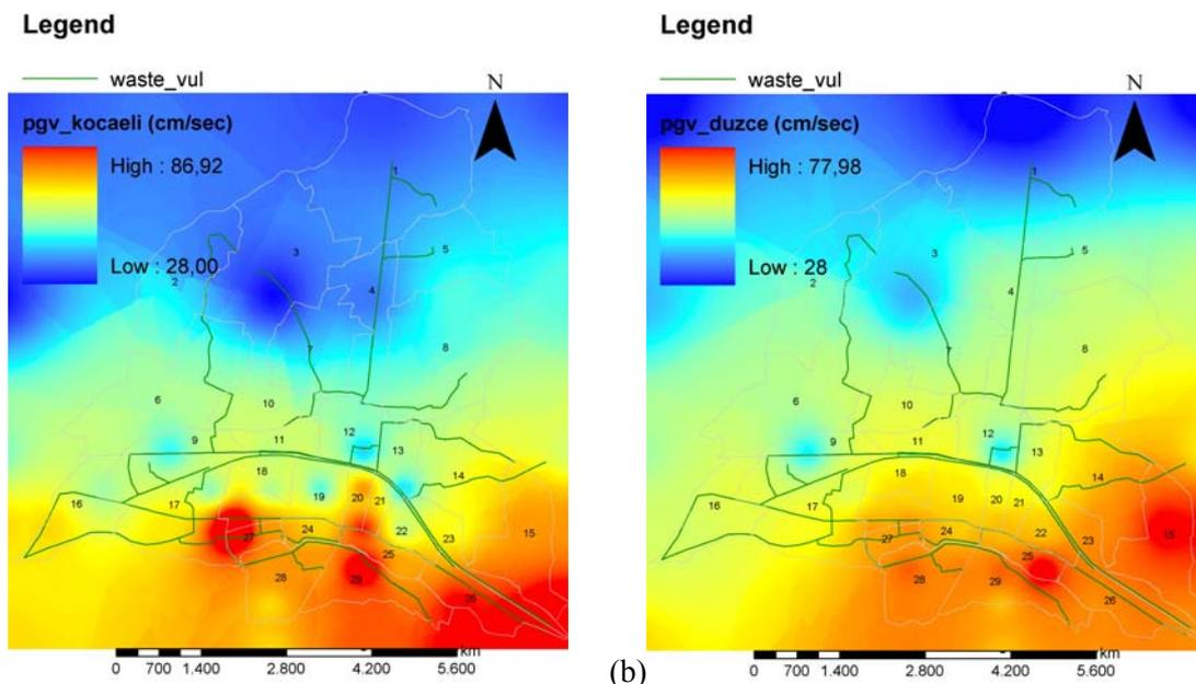
Figure 4 Spatial distribution of PGV values (cm/sec) (a) for the deconvoluted time history of Kocaeli record and (b) the deconvoluted time history of Düzce record, at the Meteorological Station of Düzce.
