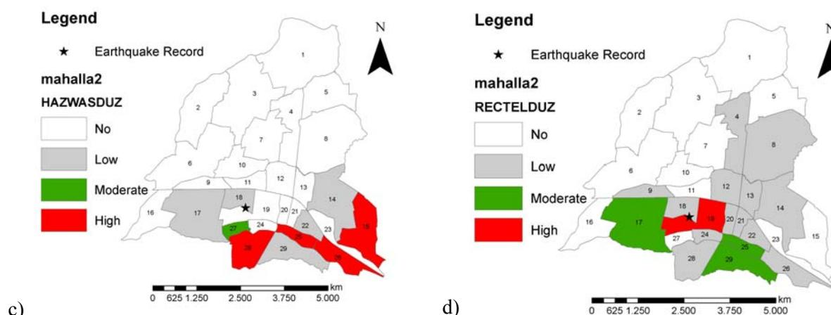
Figure 8 Estimated waste-waterpipe damages per mahalla for Kocaeli earthquake (a), after Düzce earthquake (c) and Recorded waterpipe damages per mahalla after Kocaeli earthquake (b)
