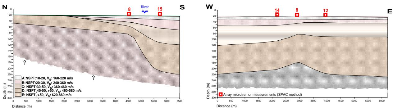
Figure 2 2D geotechnical cross-section at the NS and WE direction (in collaboration with Dr. M. Manakou).
