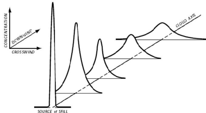
Fig 4 Gaussian distribution of gas [9]
