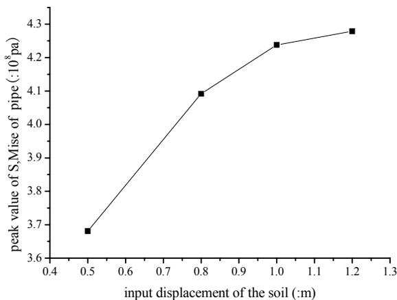
Fig 7 The influence of displacement on the max S, Mise
