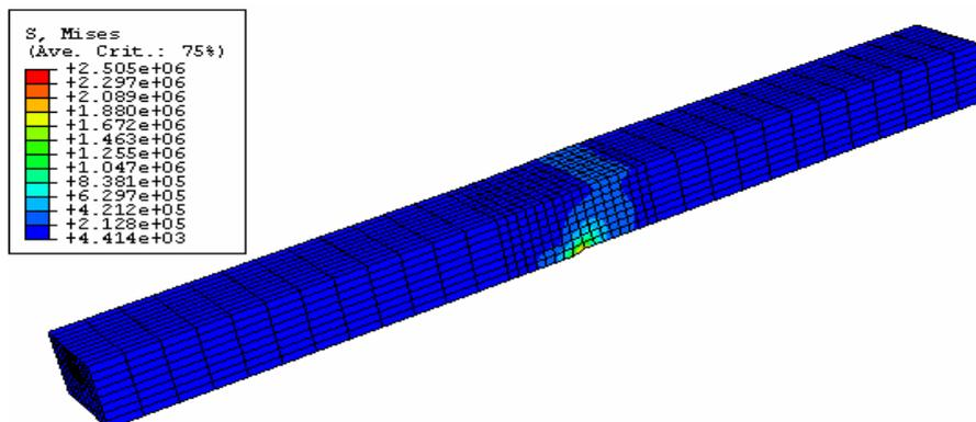
Fig 6 S, Mise of the soil around the pipeline
