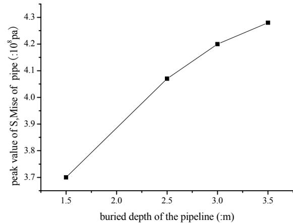
Fig 10 The influence of buried depth on the max  $S_1, \text{Mise}$
