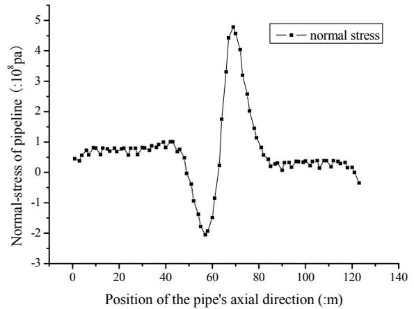
Fig 4 Normal-stress of the pipeline along axial direction
