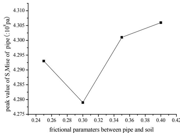
Fig 11 The influence of friction coefficient on the max  $S_1, \text{Mise}$
