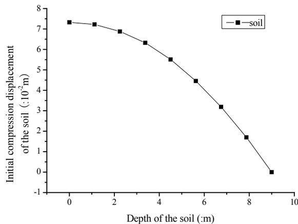
(a) initial compression-displacement of the soil
