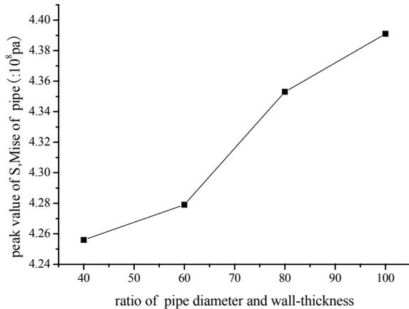
Fig 9 The influence of ratio between diameter and thickness on the max  $S_1, \text{Mise}$
