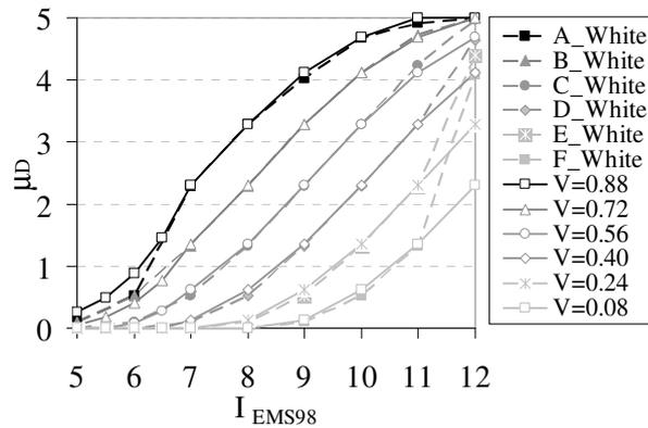
Figure 5. Curves  $I-\mu_D$  corresponding to the central “expected white” values of the definitions of the scale for the 6 vulnerability classes and corresponding parametric vulnerability curves
