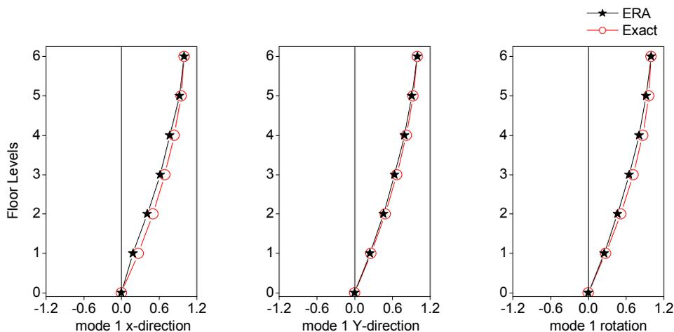
Figure 4. Mode shapes extracted from reconstructed responses using proposed modal identification method
