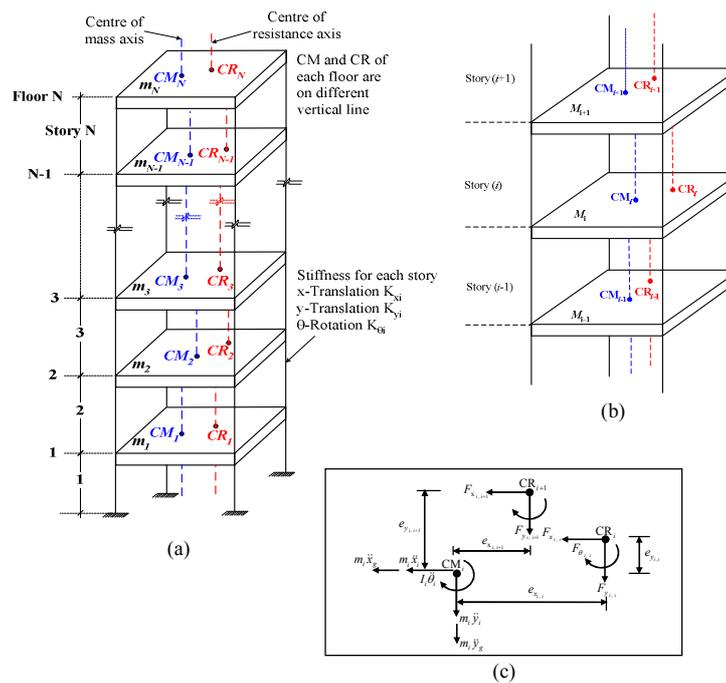
Figure 1. Torsionally coupled multi-storey building
