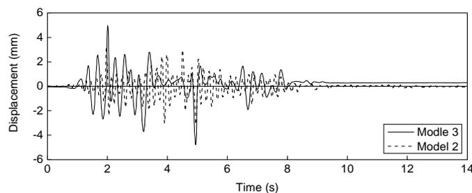
Figure 7 1<sup>st</sup>-story displacement time histories of the models under Qian'an earthquake
