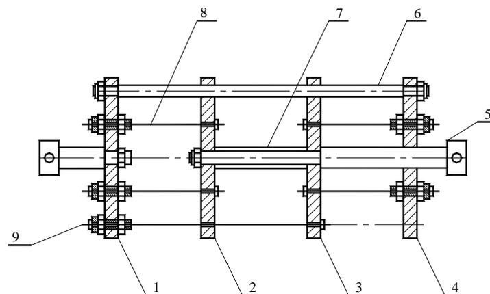
Figure 1 Configuration of the RDD
