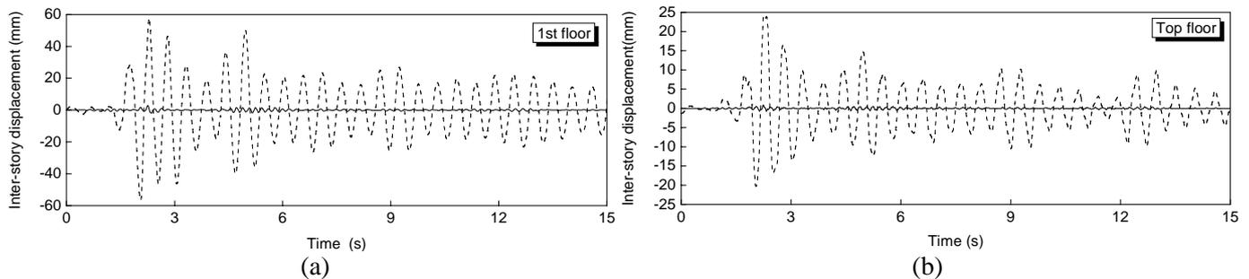
Figure 6 Inter-story displacement time histories of the models under El Centro earthquake
