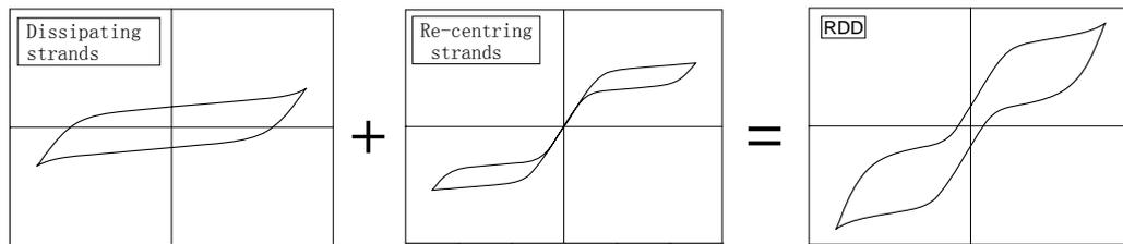
Figure 2 Mechanical behavior of the two functional groups of SMA elements
