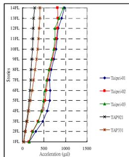
Fig.14 Building B (floor acceleration reaction chart)
