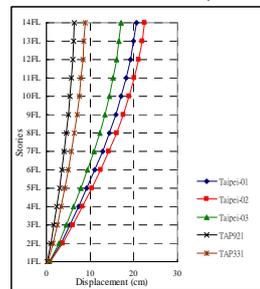
Fig.23 Building B (floor absolute displacement chart)
