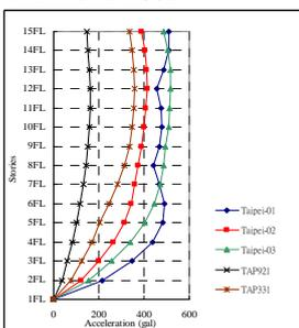
Fig.19 Building A (floor acceleration reaction chart)
