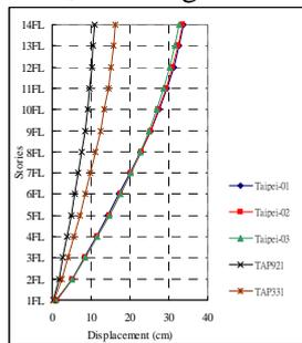
Fig.17 Building B (floor absolute displacement chart)
