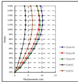
Fig.10 Building A (floor absolute displacement chart)
