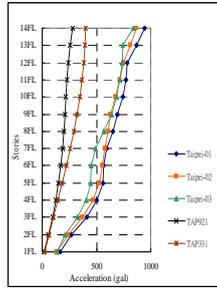
Fig.8 Building B (floor acceleration reaction chart)
