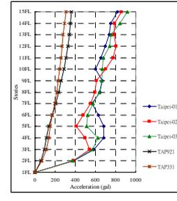
Fig.9 Building C (floor acceleration reaction chart)
