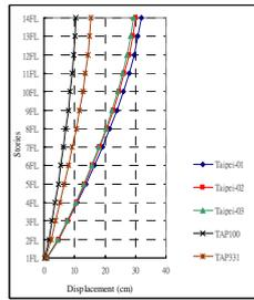
Fig.11 Building B (floor absolute displacement chart)
