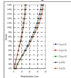
Fig.18 Building C (floor absolute displacement chart)
