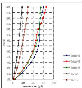
Fig.20 Building B (floor acceleration reaction chart)
