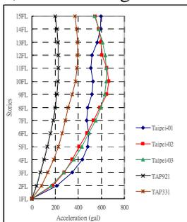
Fig.13 Building A (floor acceleration reaction chart)
