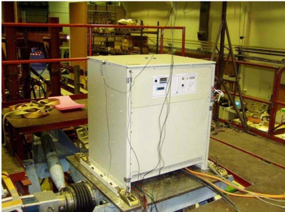
Figure 6. The EK rectifier mounted on the shaking table for testing in the Side-to-Side & Vertical directions
