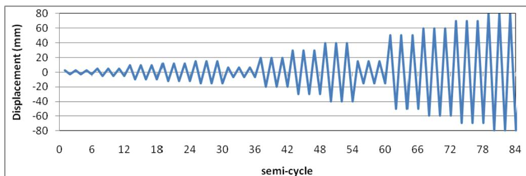
Figure 2: Target top-displacements during the tests
