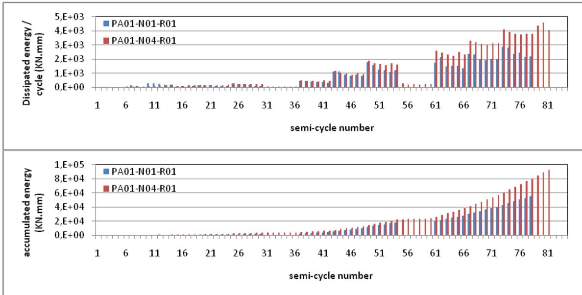
Figure 9: Dissipated and accumulated energy - Comparison between CFRP retrofit solutions
