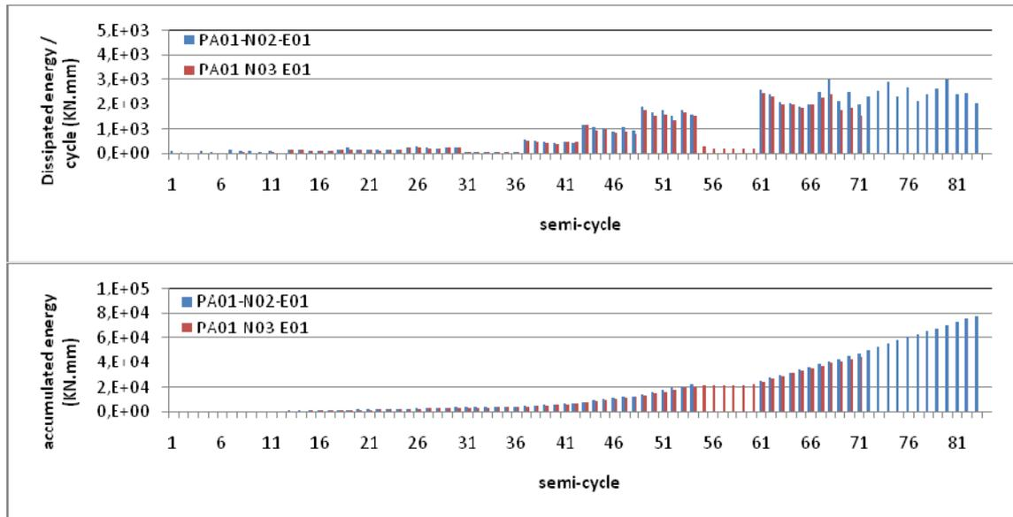
Figure 5: Dissipated and accumulated energy - PA1-N2 and PA1-N3 (“as built”)
