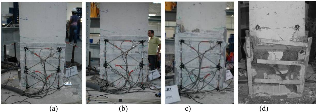
Figure 10: Damage on the retrofitted specimen PA1-N3: flexural cracking (a and c) and failure (b and d).
