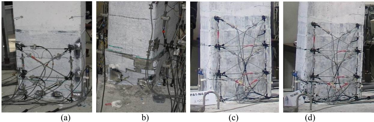
Figure 7: Damage on the CFRP retrofitted specimen: flexural cracking (a and c) and failure (b and d).
