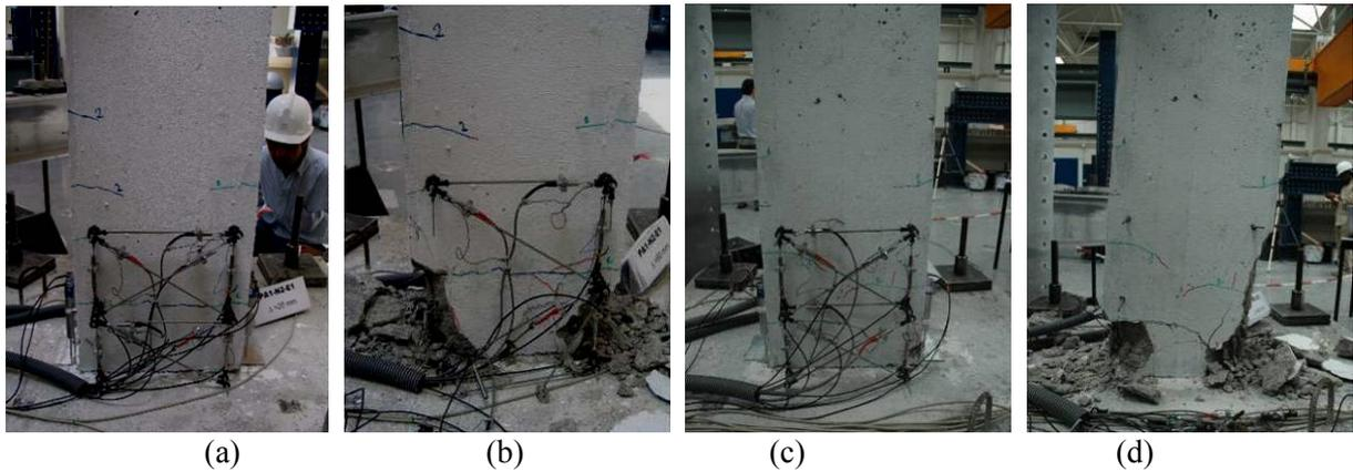
Figure 3: Damage patterns in the column PA1-N2 (a and b) and PA1-N3 (c and d).
