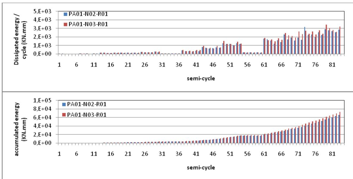
Figure 12: Dissipated and accumulated energy - Comparison between steel retrofit techniques
