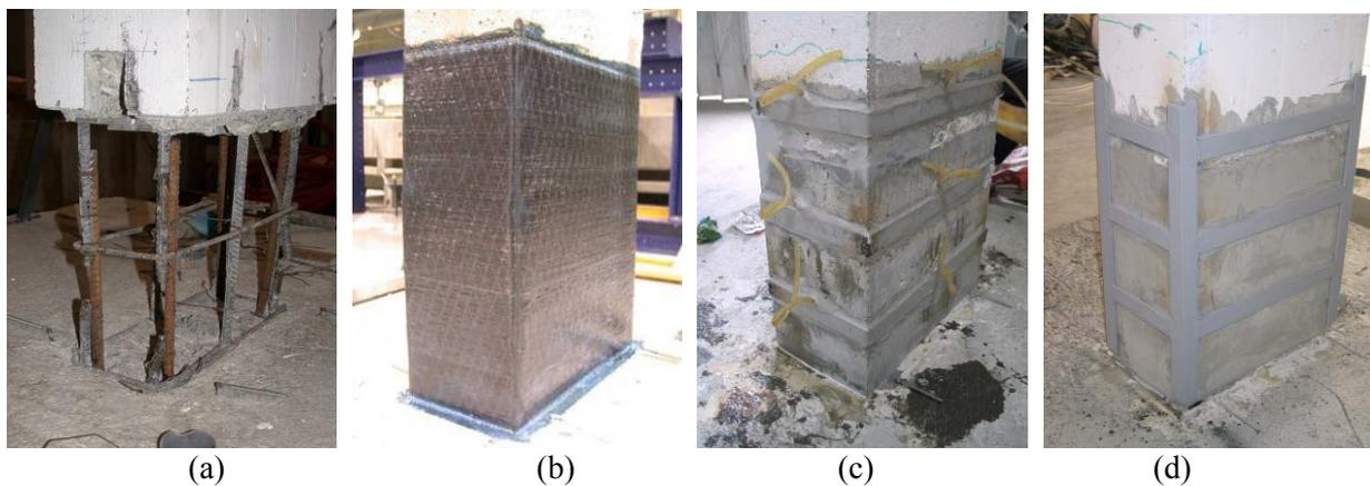
Figure 6: Lap spliced zone (a); retrofitted column with CFRP sheet jacket (b); steel plates (c); and steel plates connected by equal leg angle steel profiles (d).
