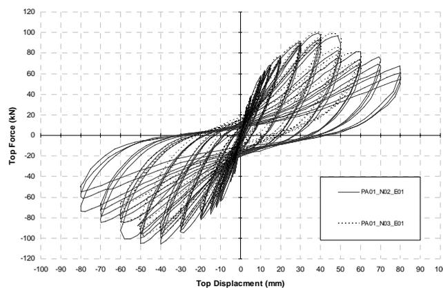
Figure 4: Experimental cyclic results of columns - PA1-N2 and PA1-N3 (“as built”)
