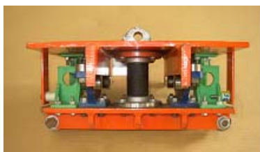
Fig.4 Base-isolation system used for the test
