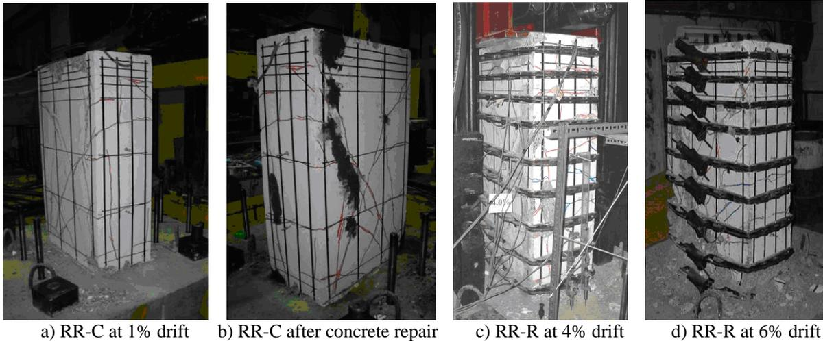
Figure 7 Damage in rectangular column before and after repair
