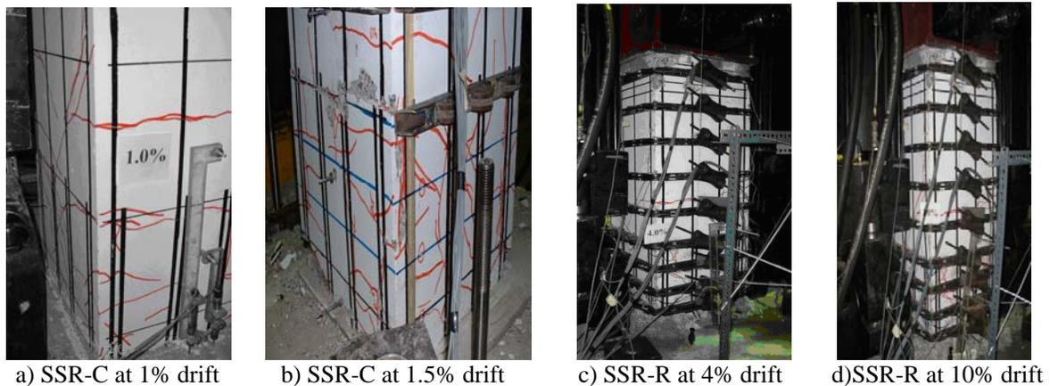
Figure 5 Damage in square column before and after repair
