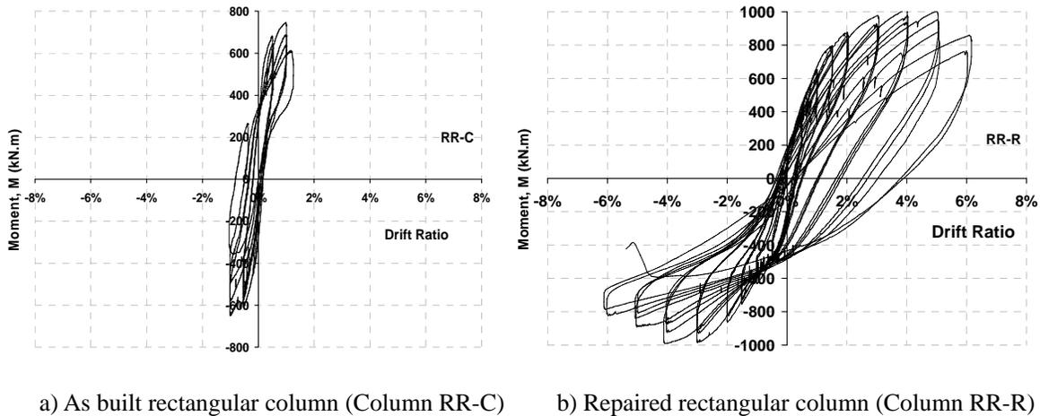
Figure 6 Hysteretic relationships for the rectangular column tested
